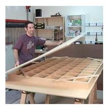
Draw lines on the skin that follow the inner grid to use as a guide as you shoot brads and drive a few screws. Use a flush-trimming router bit to cut the oversize MDF sheet to the exact size of the outer frame. Flip the torsion YOOK NAME ATTREE PROPERTY OF THE PROPERTY OF STATE OF THE PROPERTY OF THE
