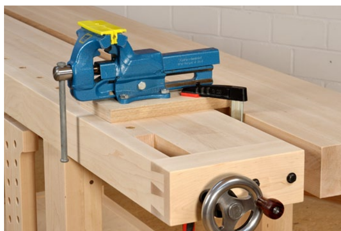
The board is simply placed loose in the slot, and can be easily removed and set aside. F-clamps can then be inserted into the empty slot between the two sections of bench top to fix work pieces or other bench top accessories in place.
