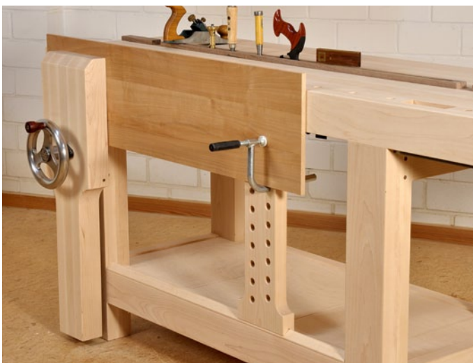
If you need to clamp longer boards in the leg vise, there is an integrated sliding deadman that can be moved steplessly between the two legs to solidly support the workpiece along its length.
