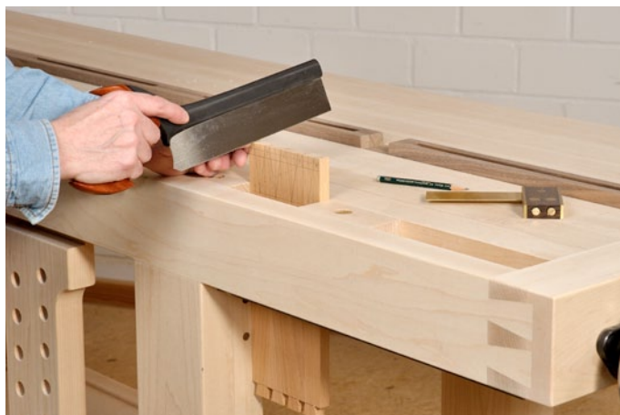
The tail vise can be used to clamp workpieces up to 310 mm wide and 45 mm thick.
