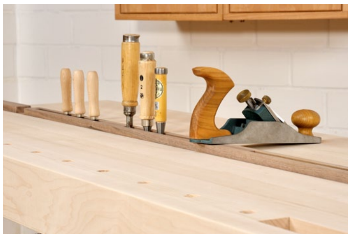
A slotted board fits the slot between the two sections of the bench top. Chisels, saws, etc. can be temporarily stored in the slots while in use, and the board makes a handy place to set planes so that their irons are protected and do not mar the surface of the top.
