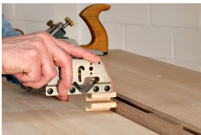
The projecting board works equally well as a planing stop, to pare the cheeks of a tenon using a rabbit plane, for instance.
