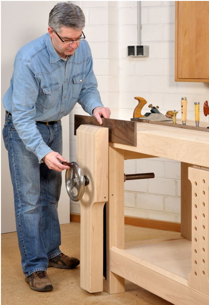
The Highlight of this bench is the extremely smooth and quickly adjustable leg vise, which is capable of very high clamping pressures.
