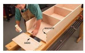
Glue and clamp the door guides to the doubled-up top and bottom. Doubling the
