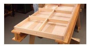
Flip the assembly and screw the bottom skin to the inner torsion frame. Then flip it back and add the top skin. Keep the torsion box clamped to the I-beams during each step to ensure that it stays flat.
