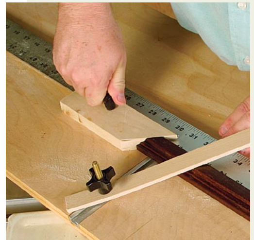
The second cut. Clamp the molding to the long fence and set the stop block at the correct distance from the blade (above). Then cut the left-hand miter (below).
