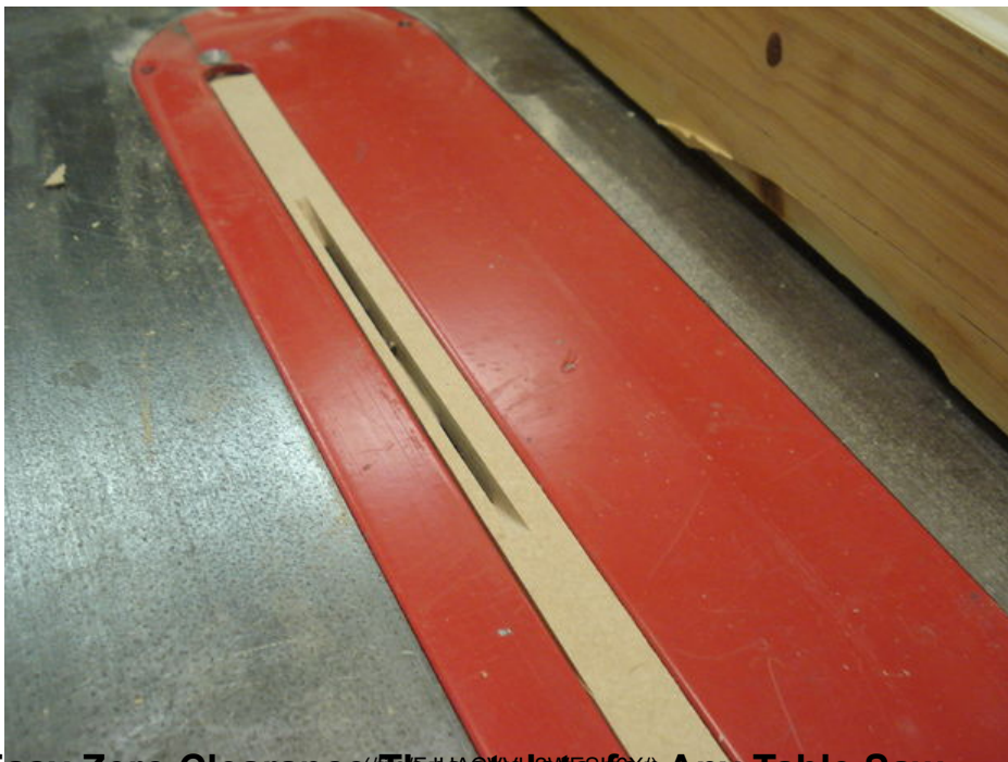
Easy Zero Clearance Throatplate for Any Table Saw by jerryjaksha (/member/jerryjaksha/) in woodworking (/explore/category/workshop/channel/woodworking/)
