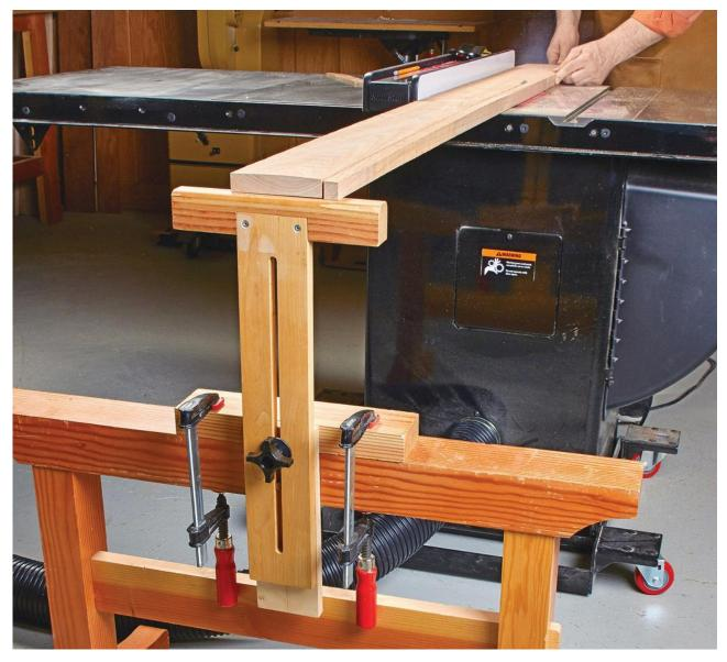
Outfeed support is nice to have on a table saw. I often use one that clamps to the rear rail of the table saw. However, on a recent playhouse build, I needed an outfeed support that was further away from the saw. So, I came up with this support that clamps on a sawhorse.
