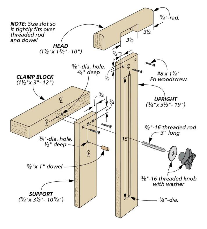
**Simple Form.** The support has a clamping block that's glued and screwed together. To allow for easy adjustment, there's a groove in the support allowing you to lock it in place with a piece of threaded rod and a knob. The head has a large roundover so workpieces slide onto it easily. A notch in it fits over the upright, and it's screwed in place. After clamping the support on a sawhorse, I can adjust the head height with the threaded knob and make my cuts.
