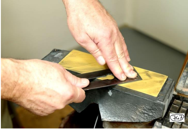
Fig. 30: Grinding the back of a plane blade on a bench stone
