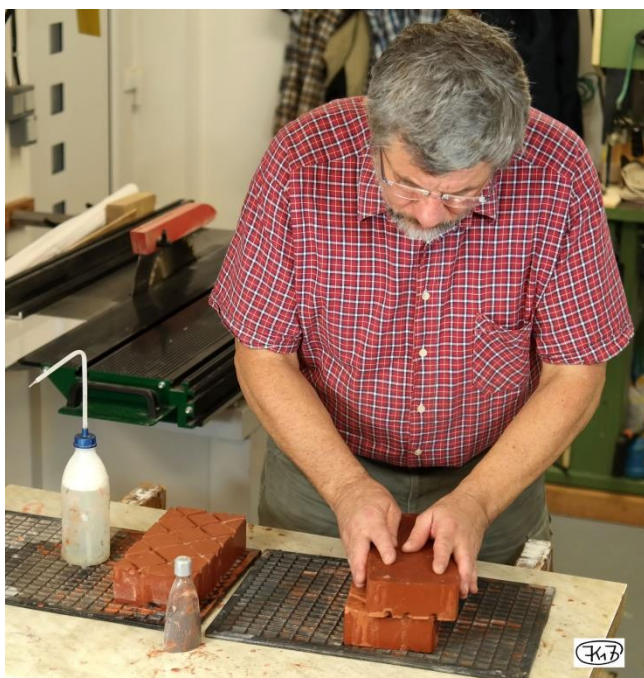
Fig. 49: Lapping the clinkers
