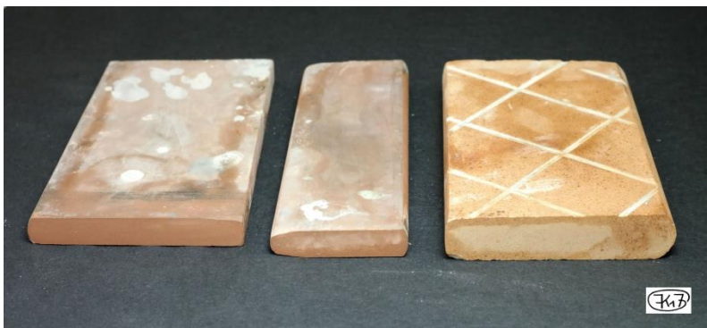
Fig. 34: Stones for working on the inside of gouges
