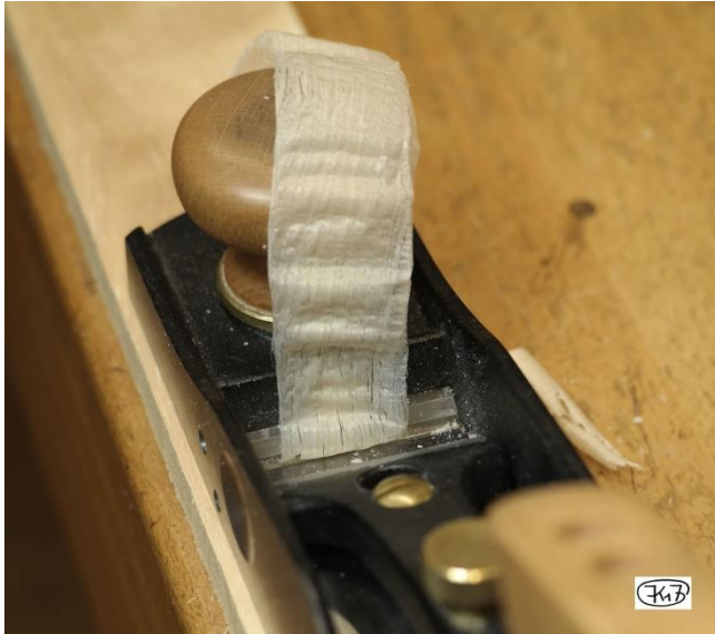
Fig. 57: Shaving produced by a smoothing plane whose blade has a cambered cutting edge
