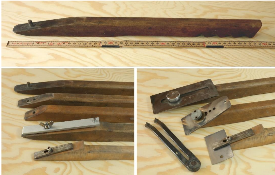
Fig. 43: Holders for plane blades above: 10° holder below left: 10°, 20° and 30° holders plus two holders for blades without a hole below right: holder with mounted blade and face spanner
