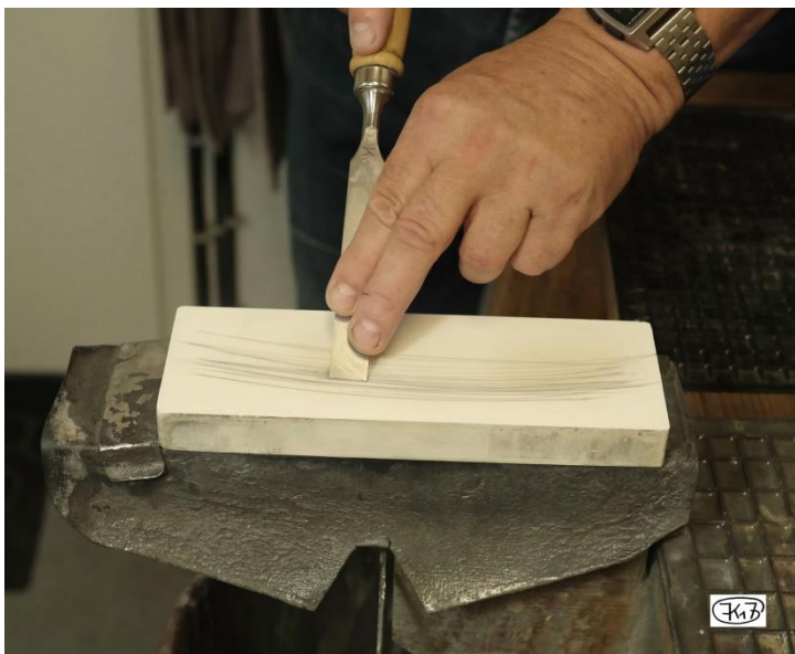
Fig. 20: Producing the microbevel
