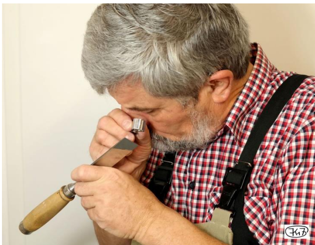
Fig. 45: Using a strong folding magnifier for checking the cutting edge
