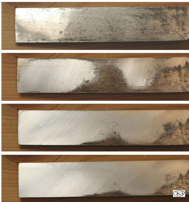
Fig. 56: Flattening a back
