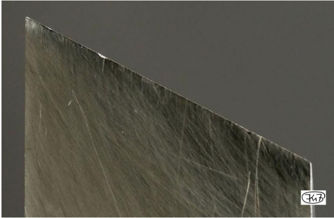
Fig. 4: Cutting edge of a 13 mm wide skew chisel
