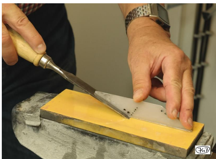
Fig. 15: Aligning the blade on the stone using an angle gauge (here: to 25°)
