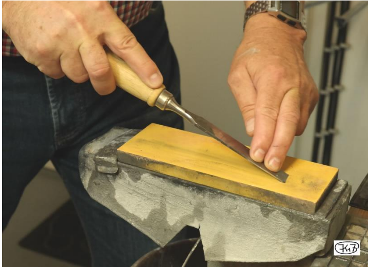
Fig. 16: Grinding a chisel blade on a bench stone
