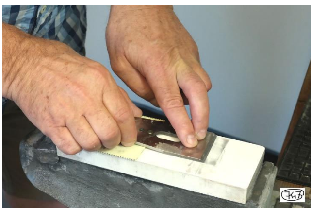
Fig. 26: Honing the back bevel
