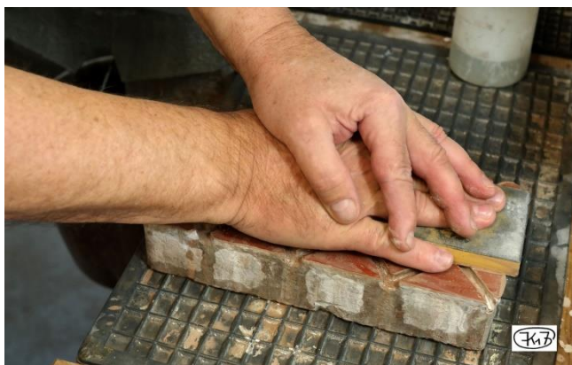
Fig. 51: Dressing a whetstone on the clinker
