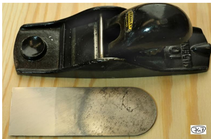
Fig. 22: Plane blade with a straight cutting edge and its plane (simple bevel up Stanley 102 plane)
