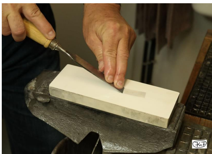
Fig. 19: Start producing the microbevel
