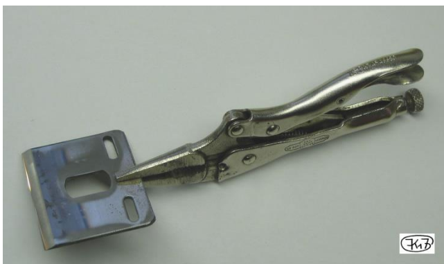
Fig. 44: Scraper plane blade, held by self-grip pliers
