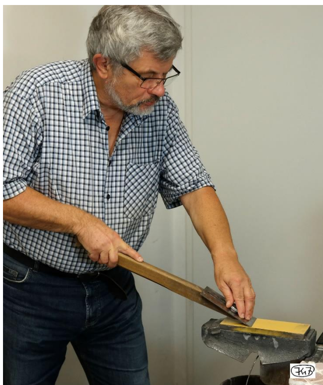
Fig. 24: Grinding a plane blade using a holder
