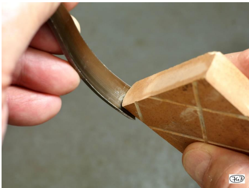
Fig. 36: Deburring the inside of curved gouge
