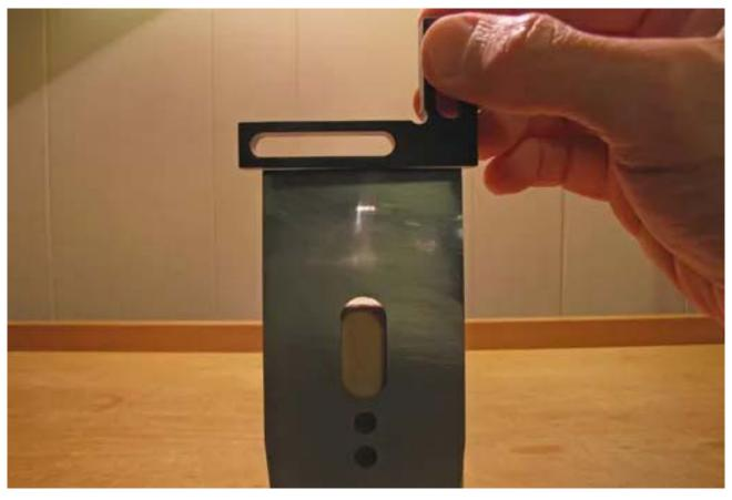
The slight curve (camber) in the edge of the plane blade is visible as a light gap against the straightedge.
