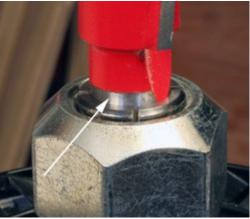
You can set some bits all of the way into the collet (left) until they bottom out but that can cause them to get stuck, occasionally in self-release collets. If you raise the bit just an 1/8" or so (right) that problem is eliminated.
