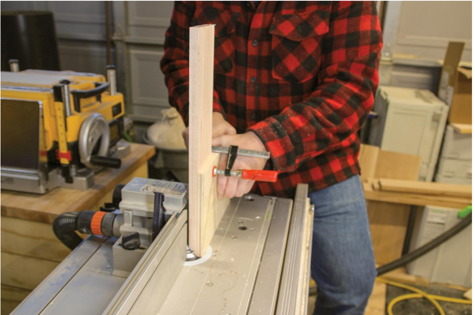
3. This simple jig, made from an offcut of drawer stock and a piece of plywood, makes it easy to keep your drawer side square against the fence.
