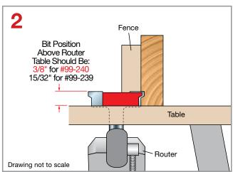
Drawer lock bits should be positioned above the router table as shown above for optimal performance.
