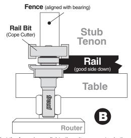
Be sure that the fence is parallel to the miter gauge track, then rout across each rail end using the same procedure described for routing the stub tenons
