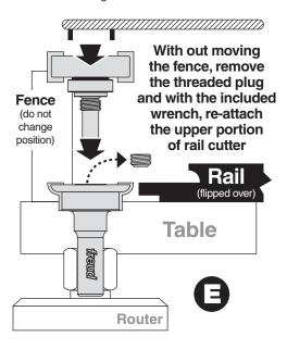
Unplug the router, remove the threaded plug and carefully thread the spindle containing the bearing and upper cutter back into the rail bit. Tighten with the spanner wrench (E). DO NOT change the position of the fence!
