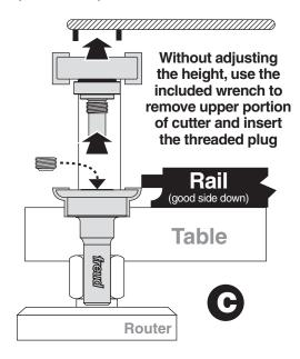
Now, unplug the router. Use the supplied spanner wrench to remove the upper portion of the cutter as shown (C). Use the router spindle lock or your router wrench to prevent the bit from turning. DO NOT change the height of the bit!
