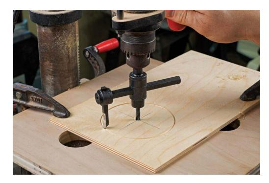
Make a template for the driver holes. Drivers need large holes, sometimes rabbeted. Use a circle cutter in the drill press to make templates, factoring in the offset between the router bit and the guide bushing you'll be using.
