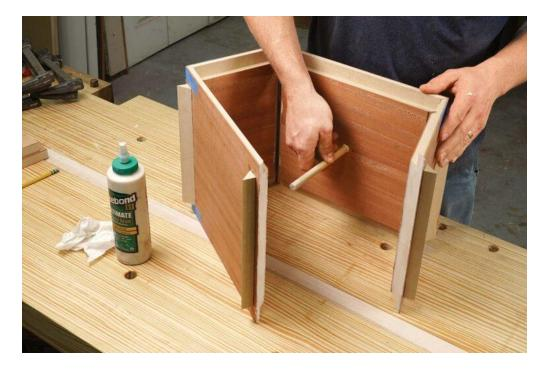
To stiffen the box, the X-Bravo design includes a dowel that connects one side to the other. Drill for this dowel ahead of time, and insert it during assembly.
