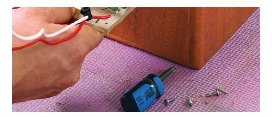
The panel slips through the larger driver hole and is screwed to the bottom of the speaker box.
