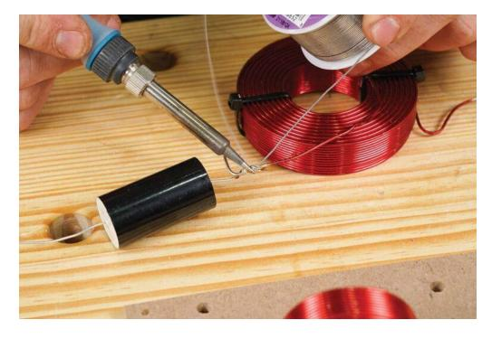
Twist the wires as shown, add flux, and solder the joints. The solder should flow along the entire joint. Check the opposite page for more soldering advice.
