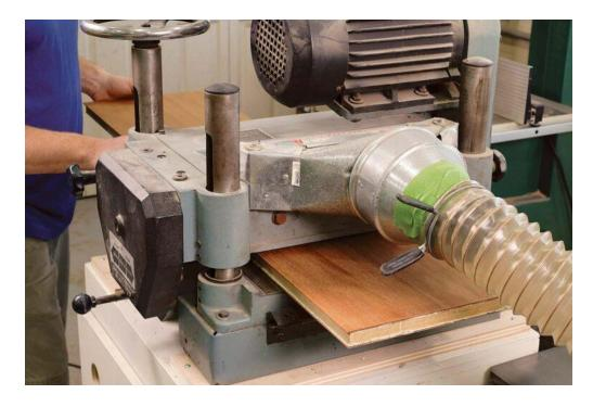
After the glue has cured, plane both sides evenly, bringing the panel down to 7/8 in. thick in the process. Use the table saw to clean up the edges.
