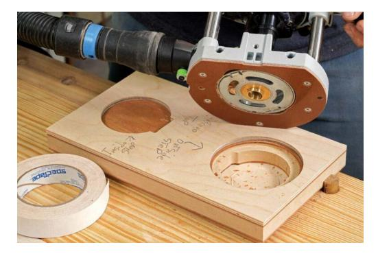
The smaller driver needs a rabbeted hole, which is notched. So this template has two different circles for routing the same driver hole. Place a sacrificial board under the workpiece, and use double-stick tape to attach the template in each position.
