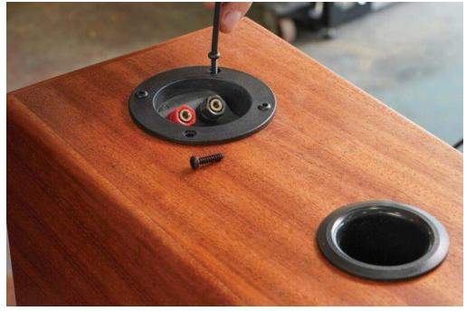
The port is simply pressed into its hole, and the speaker- **You have 1 free article remaining.** Start your FREE trial wire cup is screwed in place.
