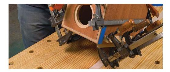
Spread yellow glue on the miter joints, close up the box, and tape the last corner closed. Then spread glue in the rabbets, add the front and back panels, and clamp lightly across the miter joints. Add more clamps to tighten the panels in their rabbets.
