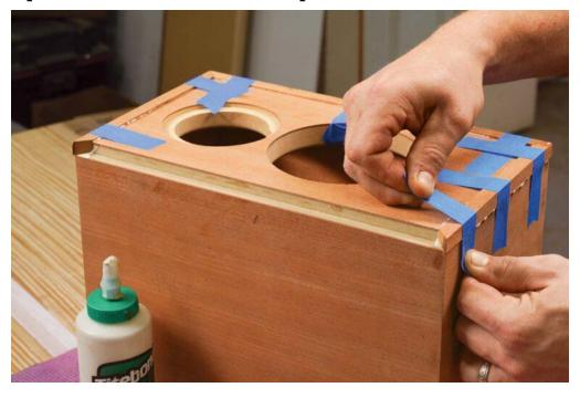
Glue in the corner strips. These are cut a bit thicker than 3/8 in. Dry-fit them to dial in the miter joints, and attach them with glue and blue tape.
