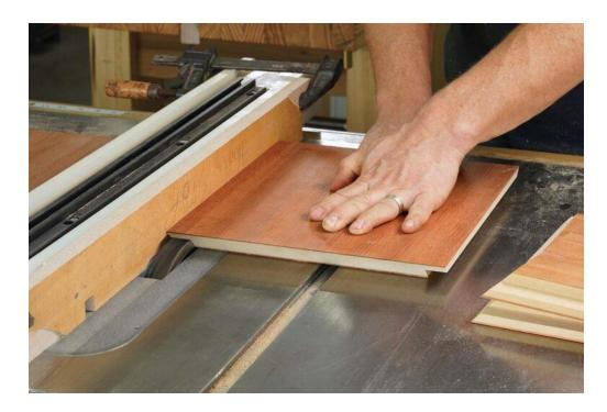
Cut the parts to exact size, and use a crosscut sled to cut the miters. Use a stop block to ensure that the cuts end right at the edges of the workpiece.
