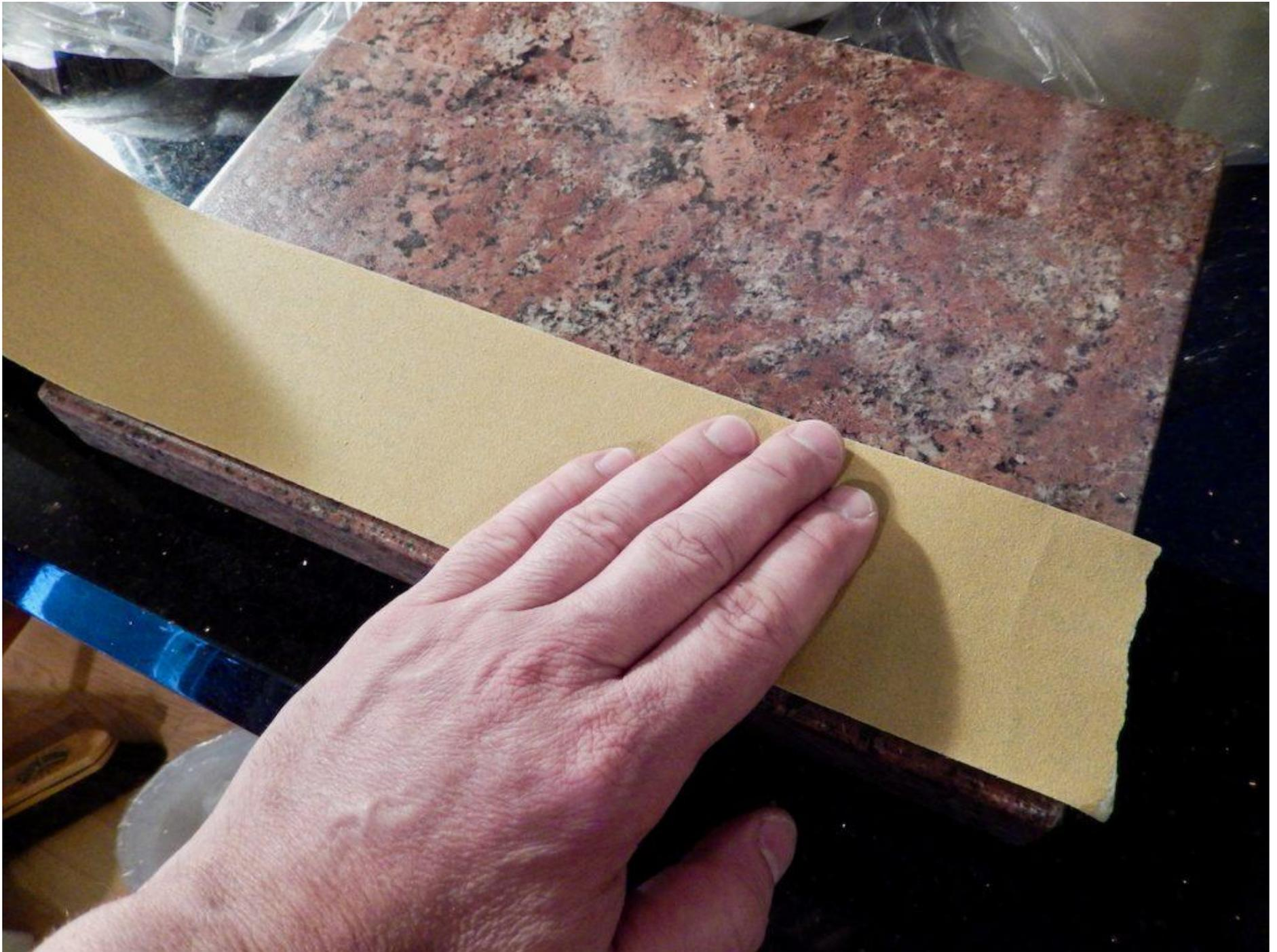
*After laying out the low-tack adhesive tape onto the stone I affix a strip of sandpaper roll over it.*
