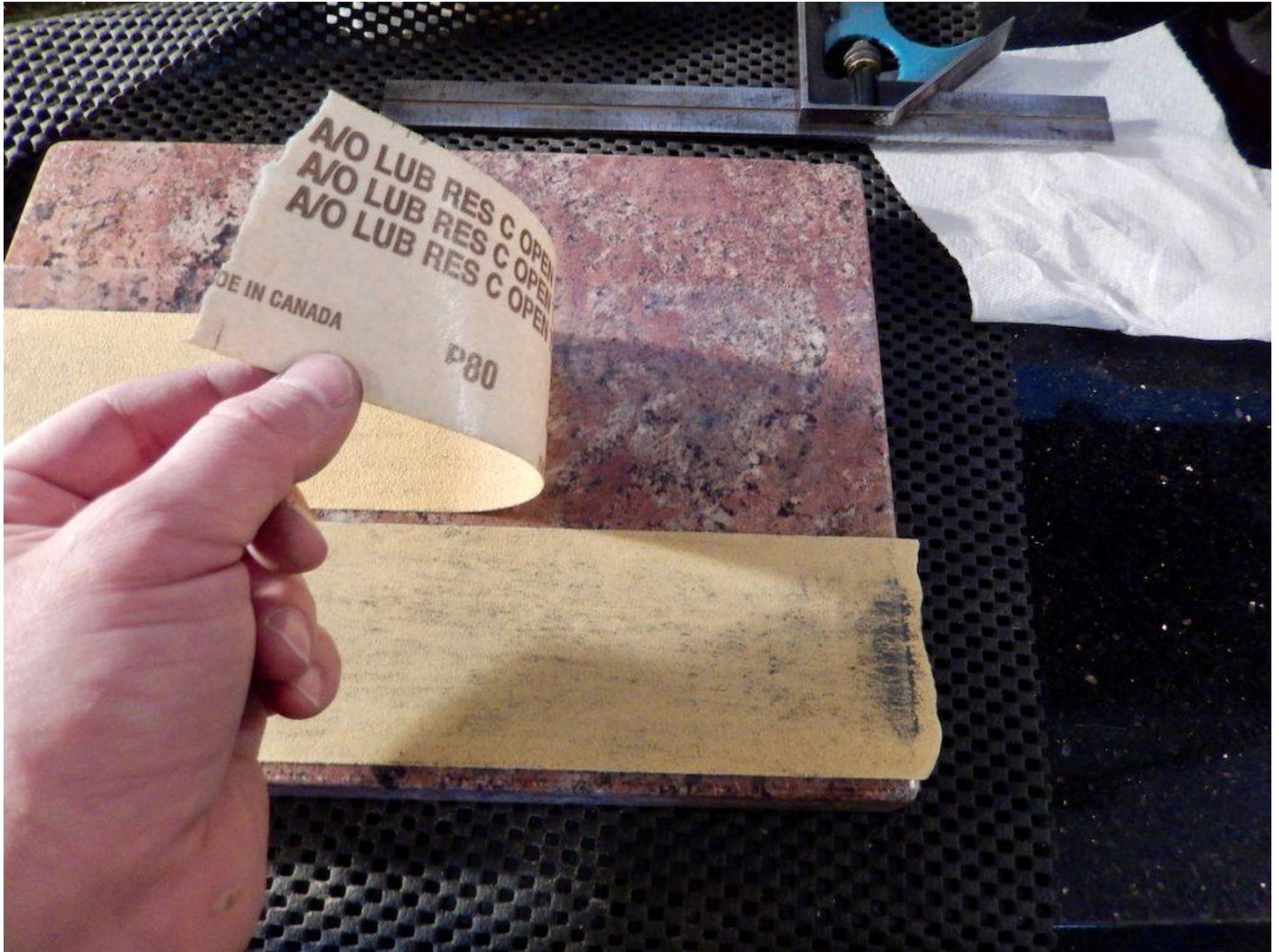
*Thanks to the Low-tack tape you can remove a worn-down strip of sandpaper and replace it with a fresh one quite easily, without the need to use a scraper and solvents.*
