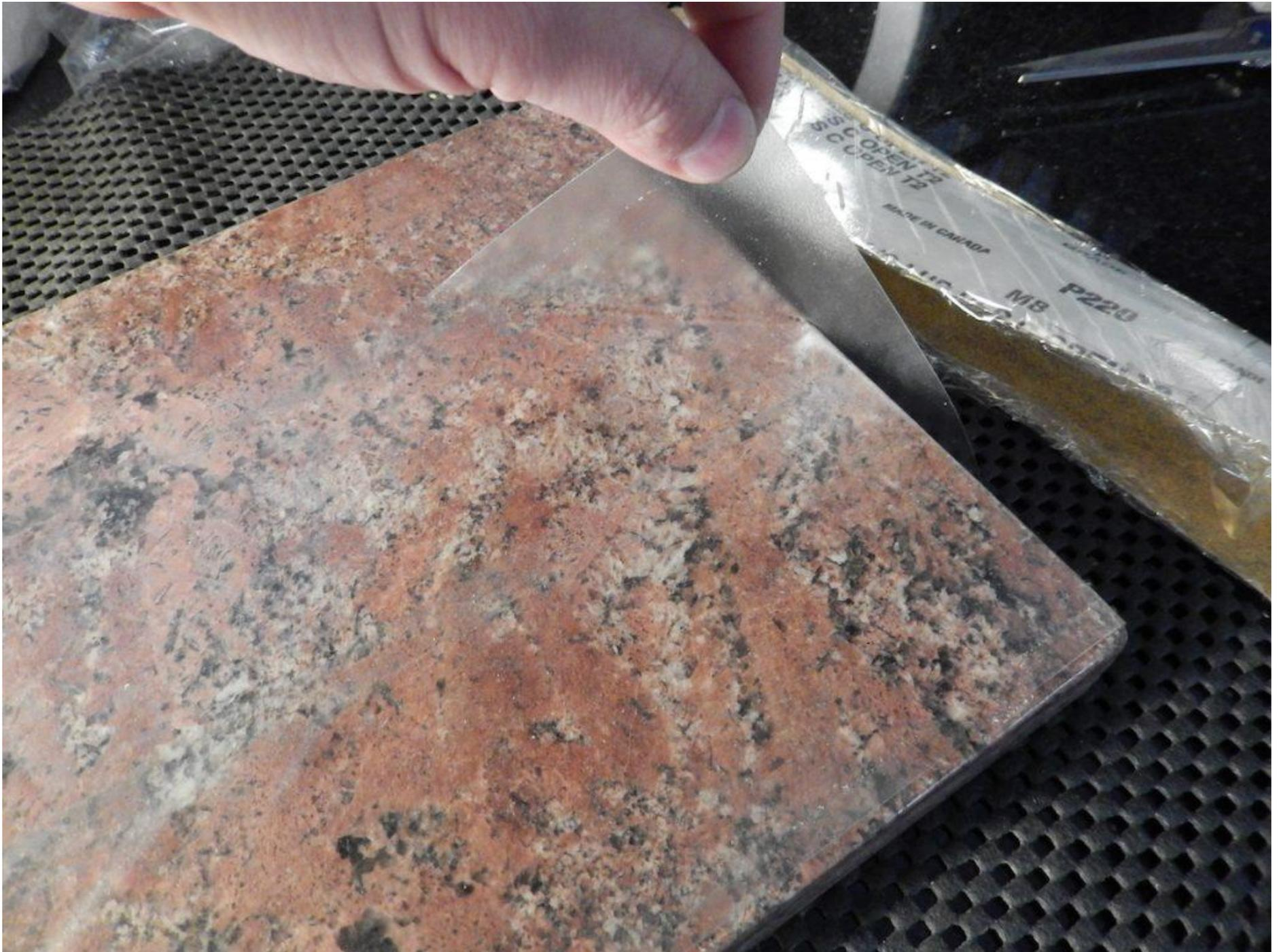
*RTape Clear Choice AT60 100 Yard General Purpose Clear Low-Tack Application Tape is a great liner for your lapping surface that protects it but also makes it very easy to peel the sandpaper strips during, and after the lapping concludes.*
