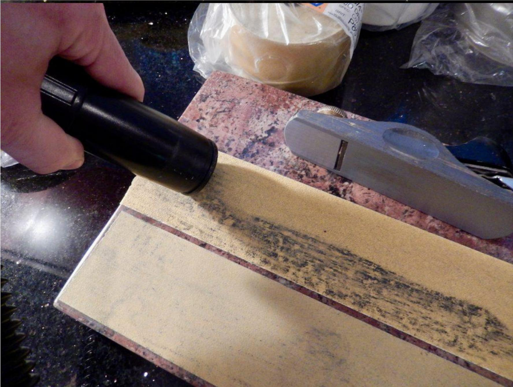
Remember to check for flattens using a straight edge and the sole sharpie serpentine line technique.
