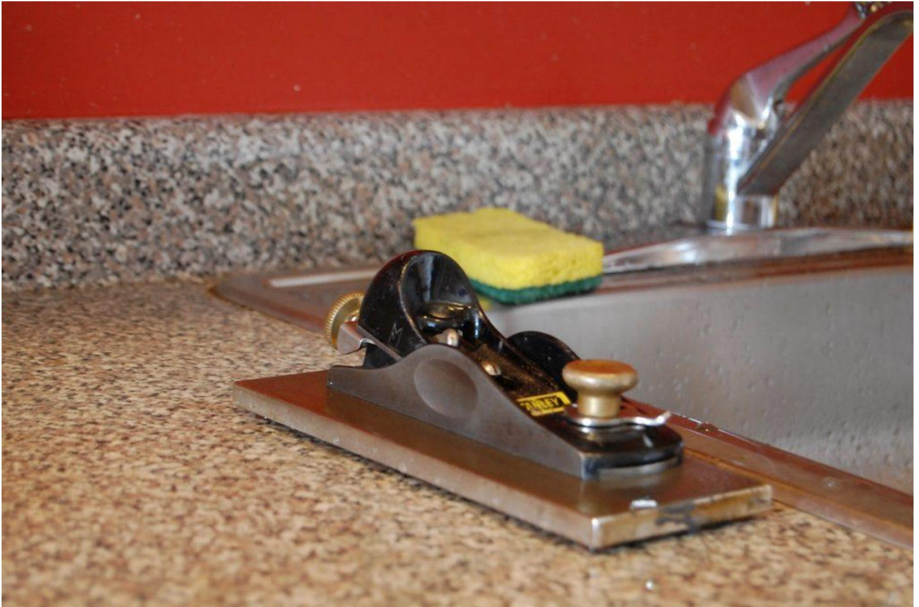
*Wet the stone with water or other particle clearing fluid and start shuffling the plane back and forth on the entire surface of the stone.*
