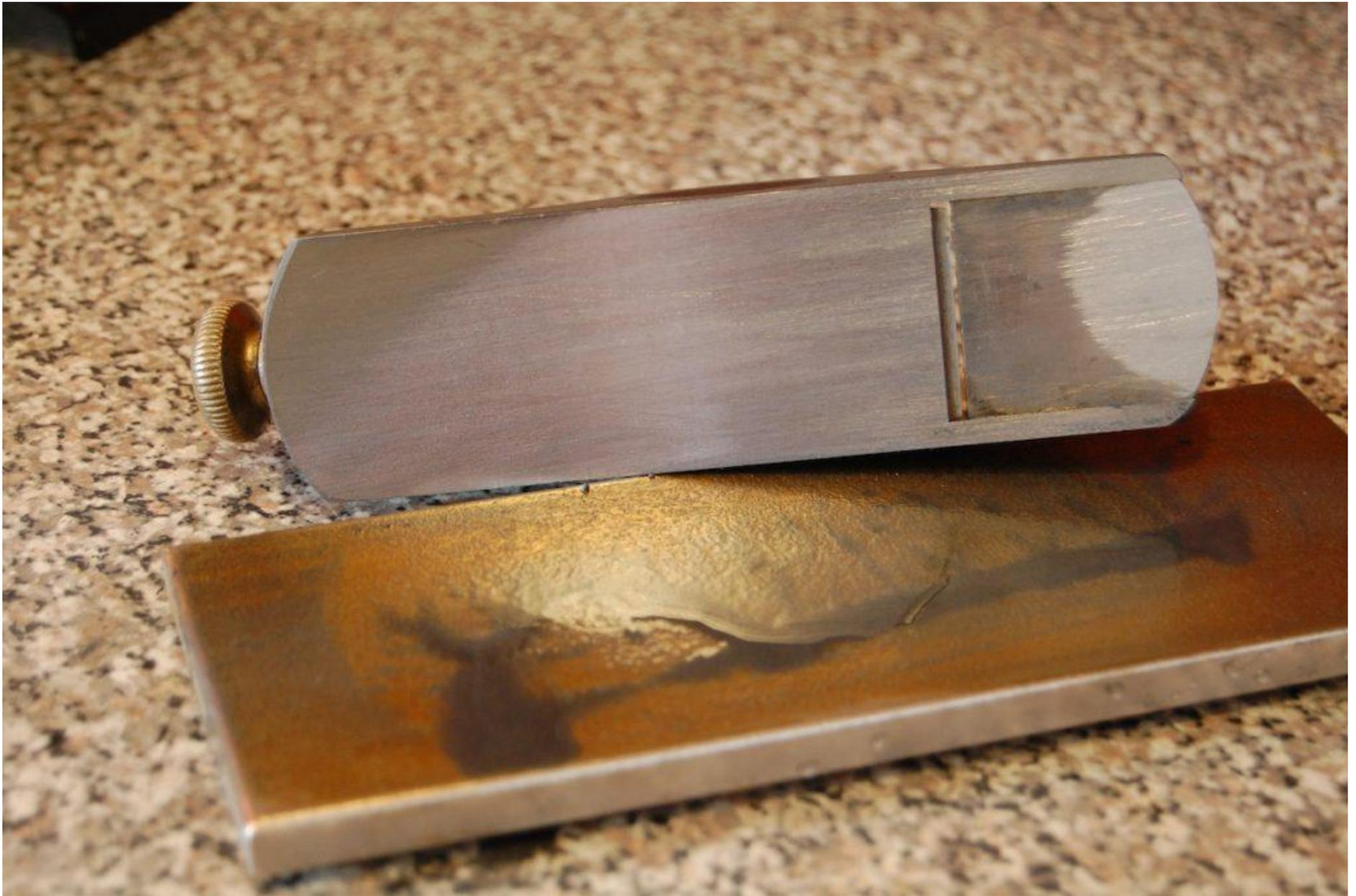
*Lift the plane and check your progress. The plane in this picture is gradually flattened. The gray-yellow furnished surface is making way for a fresh and flat silvery cast-iron surface. If the sole is covered with rust or is tarnish, I don't bother drawing a sharpie serpentine line on it. If the plane is fresh out of the box and exposes a shiny metallic sole, I would reach out for a black sharpie pen and mark the underside with serpentine or crisscross lines.*
