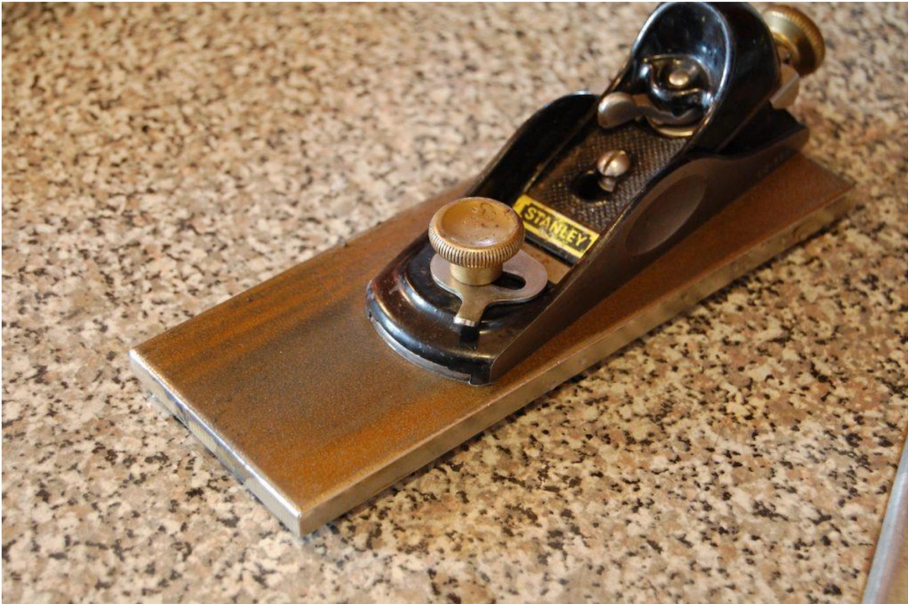
Much has been written about the importance of a true and flat plane sole as a key to achieving optimal results during planing. Premium planes come with a very flat sole, do not need any interventions, and are ready for work straight out of the box. Unfortunately, this is not the case with second-hand tools such as planes bought in flea markets or on eBay, and new inexpensive
