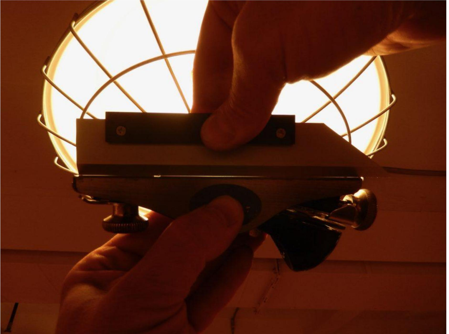
*Place a straight edge against the sole and hold the plane and the straight edge in front a source of light to see the low and high point that needs to be unified into one true plane.*
