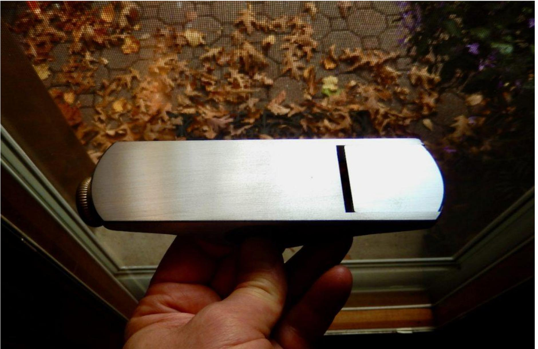
*The plane's sole is flat and true when all the high surfaces were reduced and unified into a true plane.*
