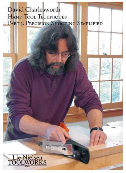
So I start with my out with a board I've trimmed on our out-of-whack (surprise!) miter saw. It's out by a couple degrees. I put plane in the track (I always use a heavy plane with an iron that is sharpened straight across). Then I put the jointed edge of the board against the shooting board's fence and show the wonky end to the plane's sole. That shows me which corner is high and which corner is low.
