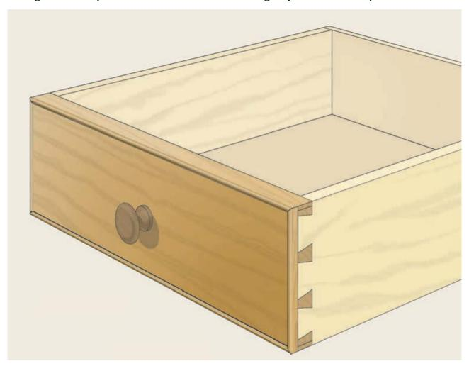
The chest of drawers on page 32 features cock bead (bead that stands proud of the surface) framing the drawer openings in the case. The applied bead adds pleasing depth and detail to the flat front of the case. In this instance, the beading was simply mitered to fit inside the drawer openings and then glued in place. This is a commonly used, tried-and-true method of adding cock beading to a project.
