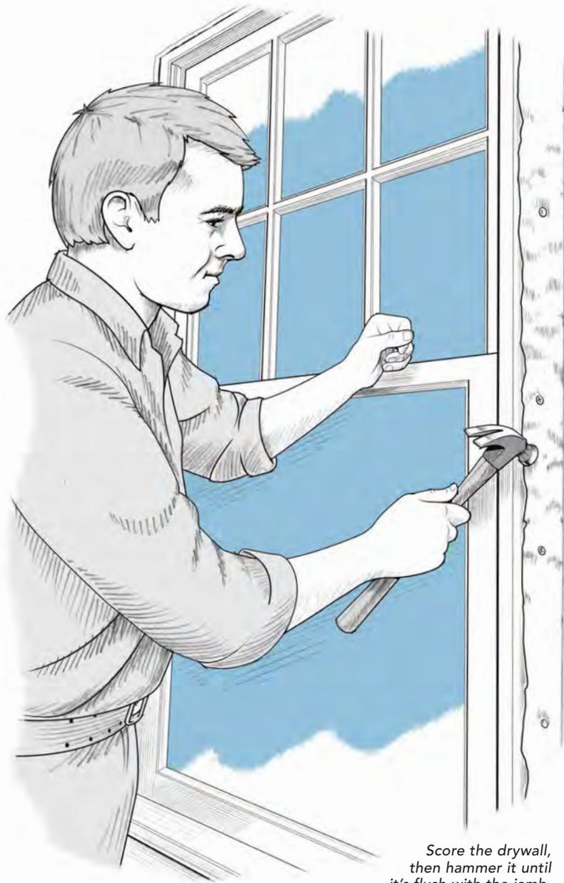
Score the drywall, then hammer it until it's flush with the jamb.
