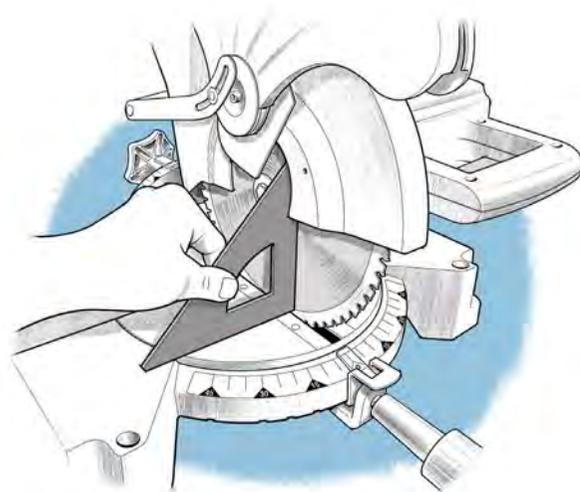
Set the bevel by squaring the blade perpendicular to the saw's table.
