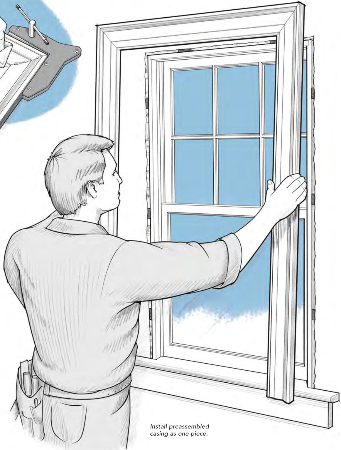
*Install preassembled casing as one piece.*
