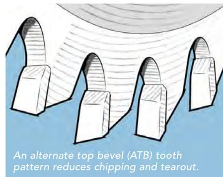
An alternate top bevel (ATB) tooth pattern reduces chipping and tearout.
