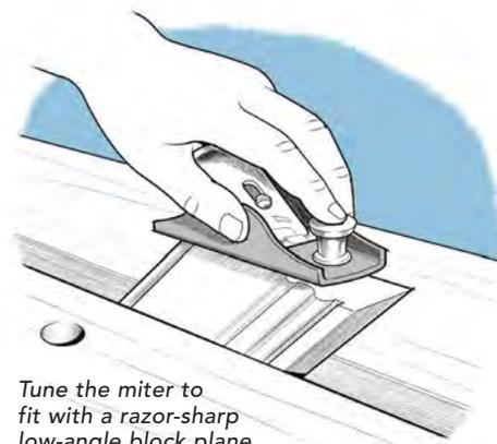
Tune the miter to fit with a razor-sharp low-angle block plane.
