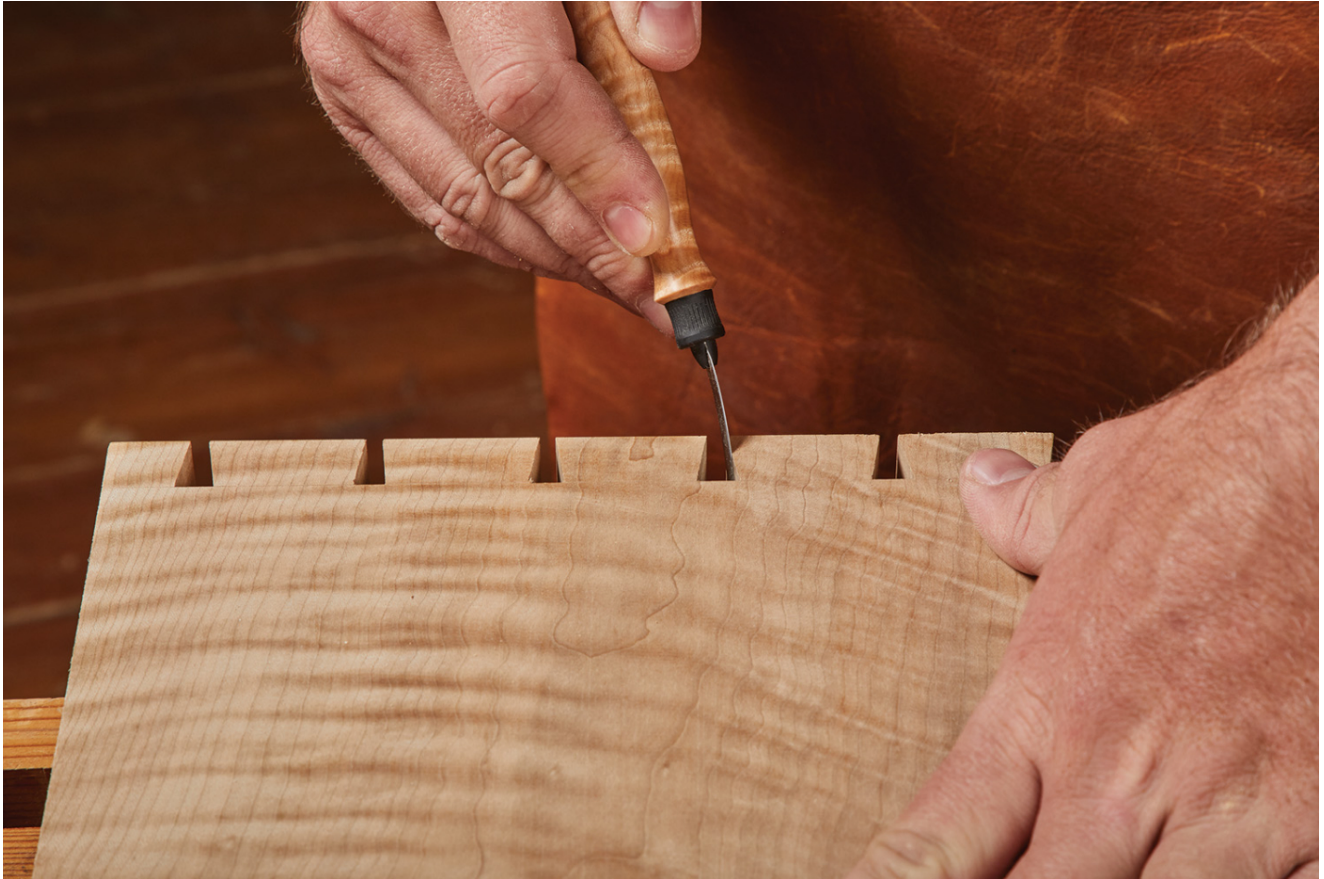
14 A flexible knife helps accurately transfer the marks across boards.
