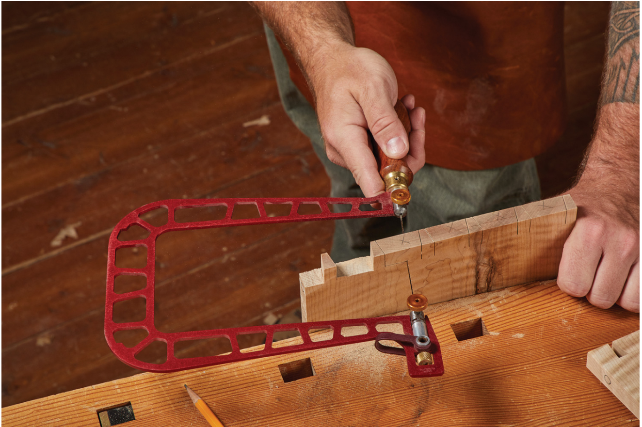
16 Angle the fret saw to remove the pin waste.
