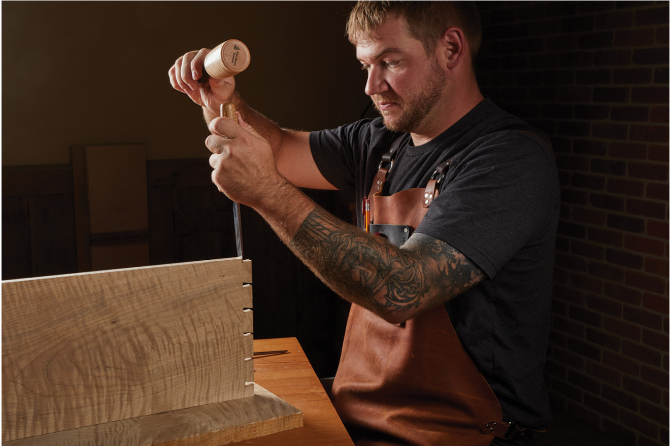
11 Stand the board on edge and chisel down the shoulder.
