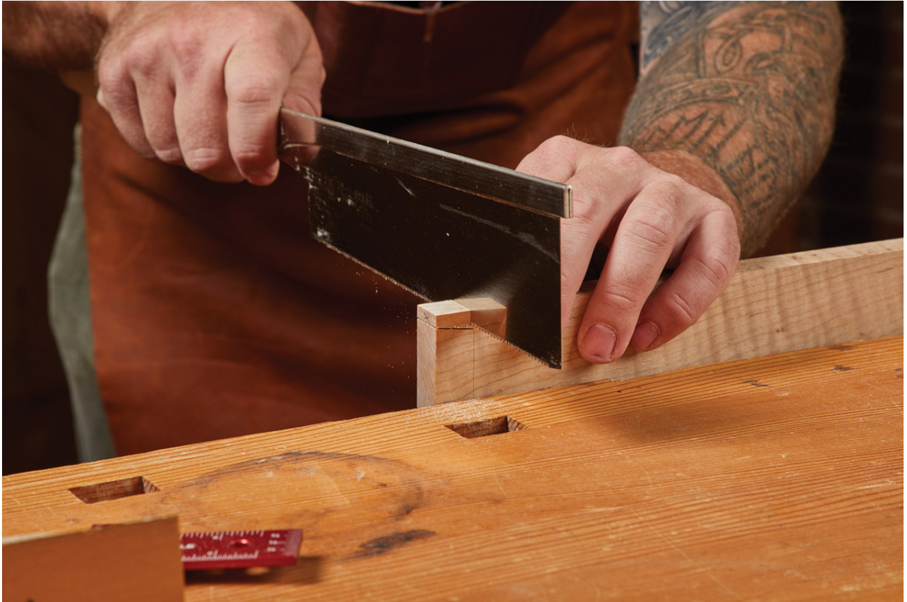
8 Cut away the waste on the shoulder of the tail board.
