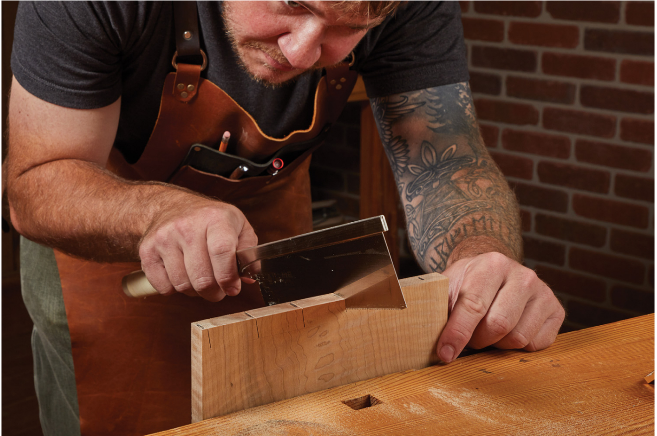
6 Drop the heel of the saw to bring the cut to the baseline.
