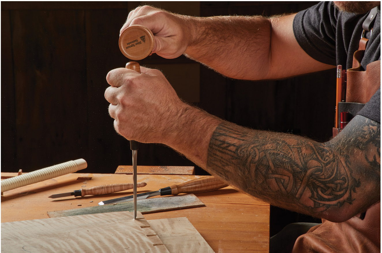
11 Stand the board on edge and chisel down the shoulder.
