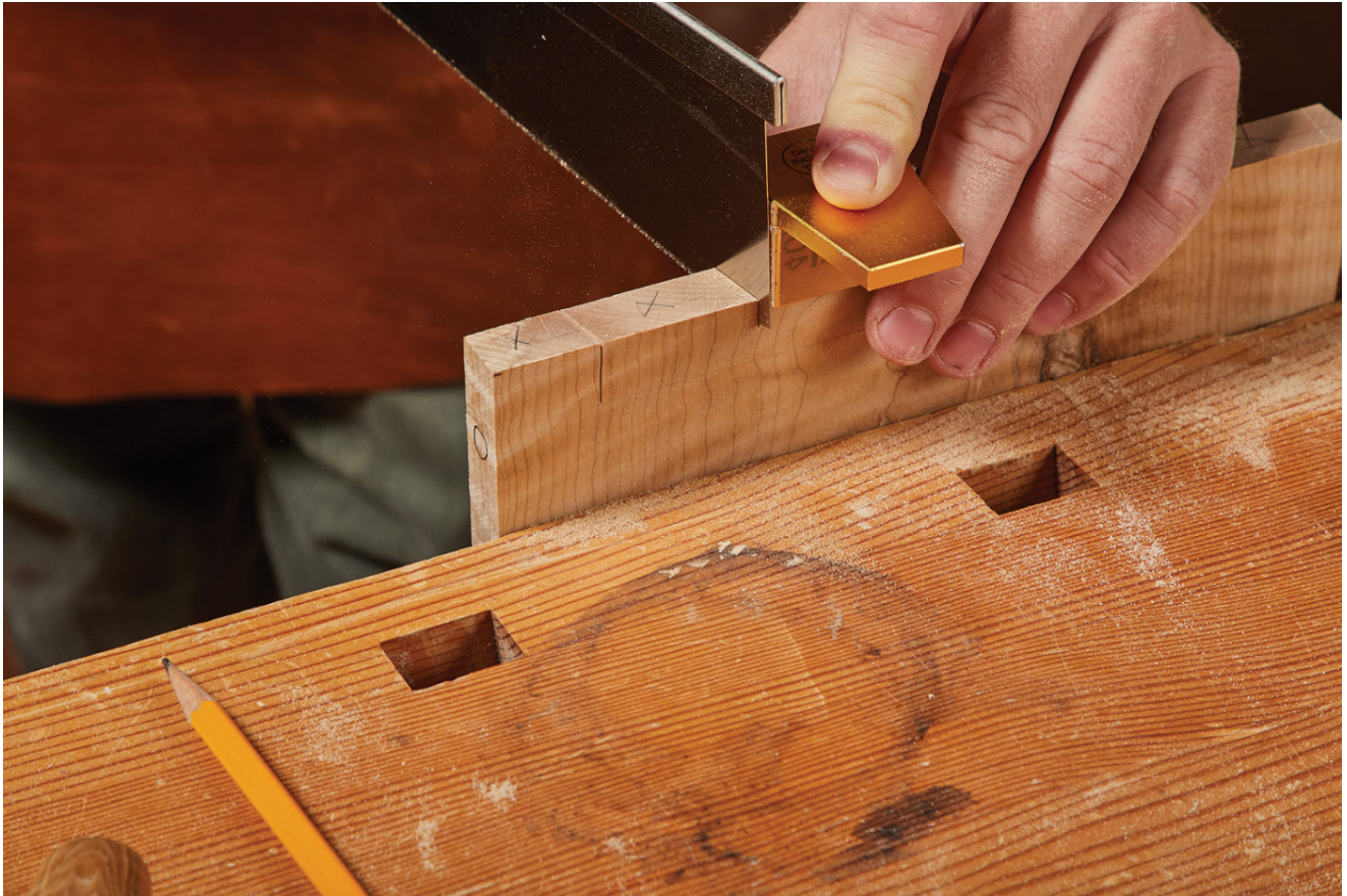
15 A dovetail guide keeps a consistent angle between tails and pins.
