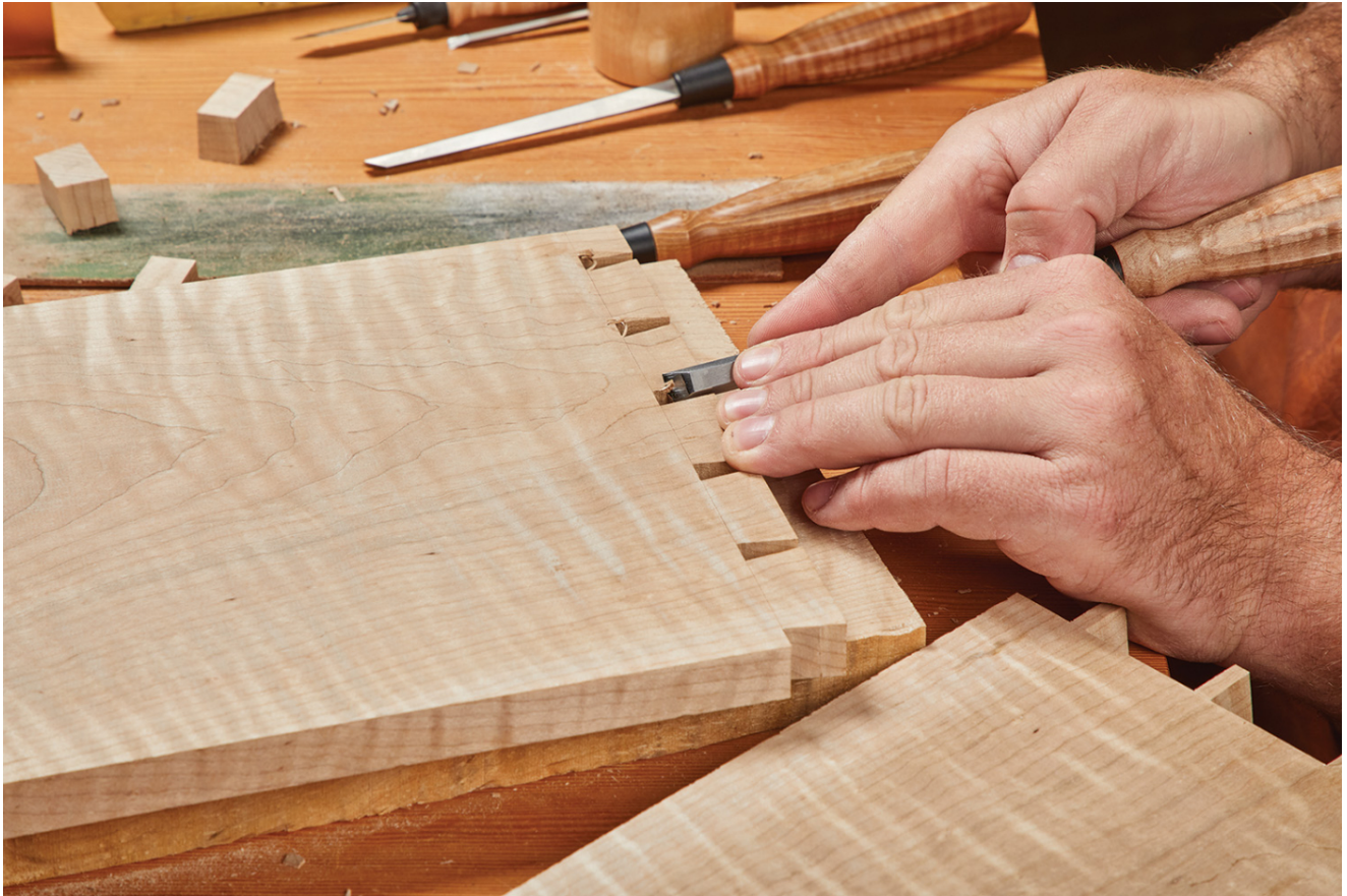
17 Chamfering the inside edges of the joints helps avoid corners snagging and keeping the joint apart.
