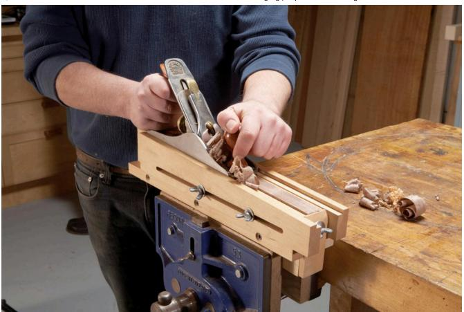
Achieving exact thickness is really important when making splines to reinforce box corners. The splines have to fit perfectly in the saw kerfs —a few thousandths of an inch one way or the other can make a big difference.
