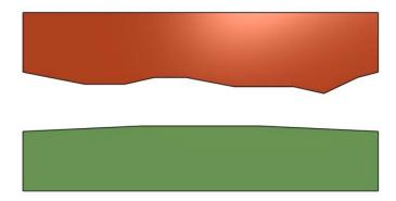
At the completion of this step, all three plates are of roughly equal flatness, but one (Green) is convex and the other two are concave:
