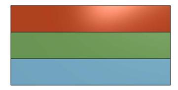
It's also worth noting that, although this yields great precision "from nothing", Joseph Whitworth later improved upon the technique by utilizing engineer's blue and hand scraping, as mentioned previously. Engineer's blue alone would be an instrumental improvement over using no indicator - with the blue, it's easy to see which areas have, and haven't been, scraped.
