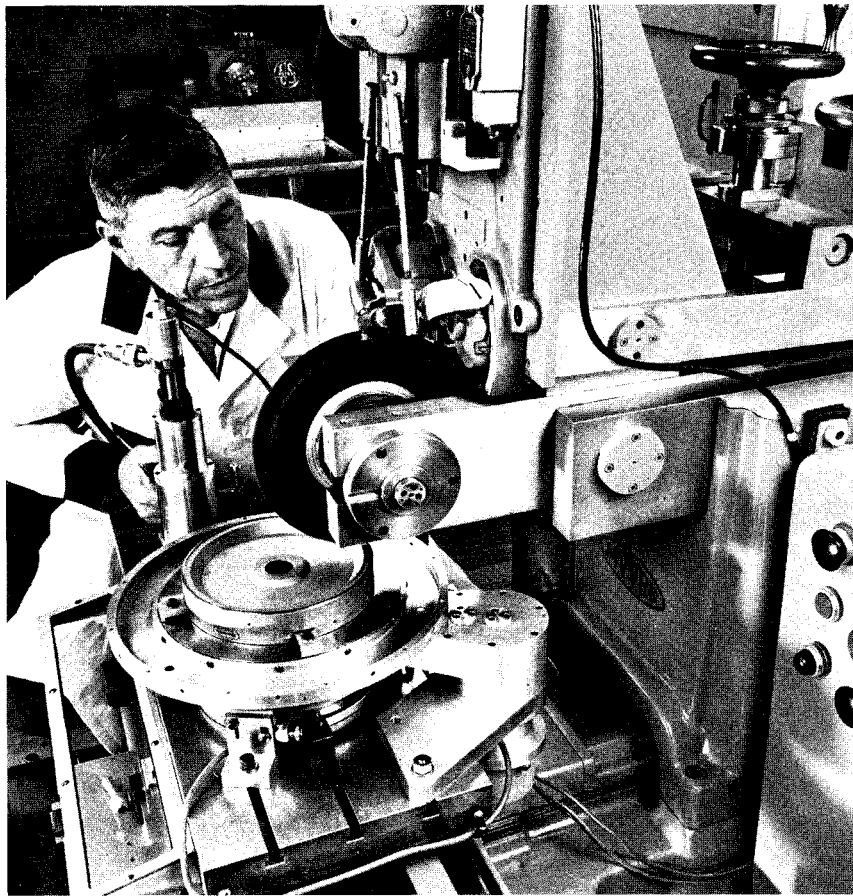
FIG. 376—To attain the \pm 0.1 second accuracy of the 1440 Index, the teeth of each member must be ground as accurately as possible, prior to lapping. At this stage, a measuring machine base is
