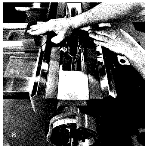
screw dial arc cut on the jig borer with a .003 inch [0.076 mm] wide saw, and the spacing is controlled by a rotary table of \pm 2 seconds accuracy. No. 5—Pitch diameter of the lead screw is inspected for uniformity. No. 6—The lead screw is inspected for concentricity of the pitch diameter to the bearing diameter.
