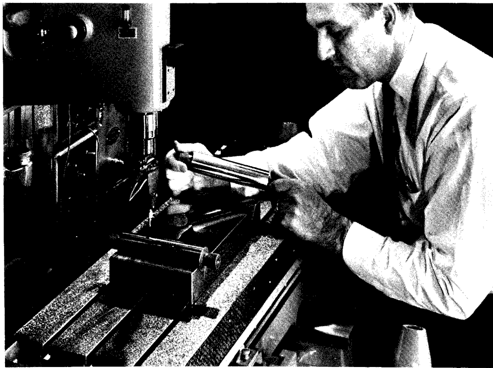
FIG. 44—The Universal Measuring Machine is the most accurate method for establishing center-distance of double V masters.
