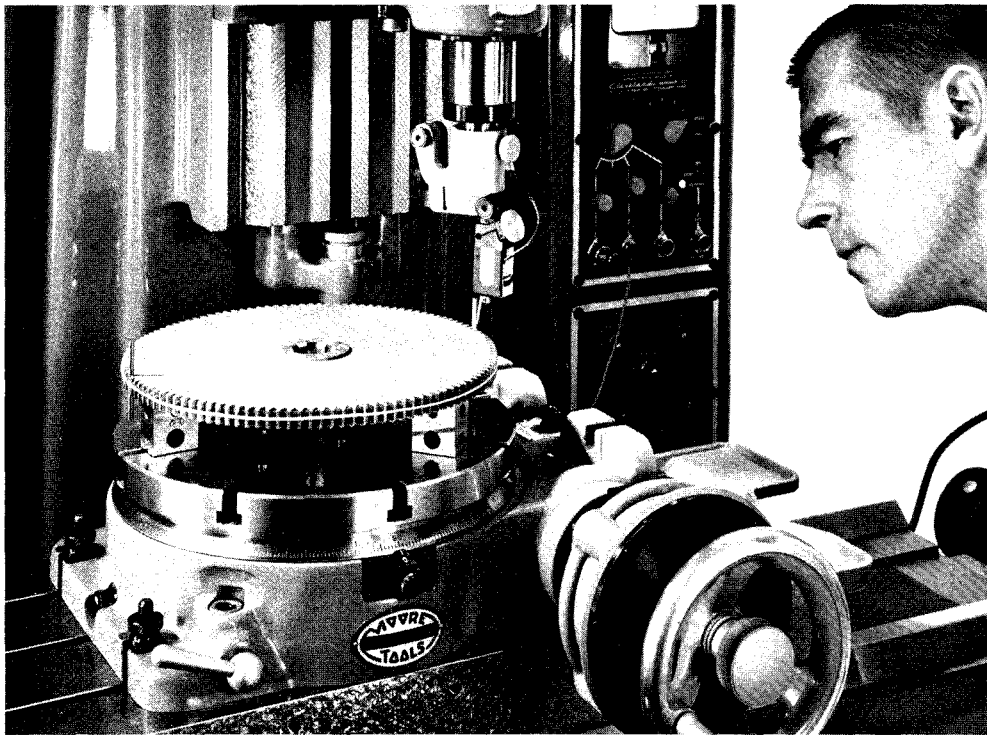
FIG. 520—Angular spacing of gear teeth is most truthfully inspected when the Rotary Table is used in conjunction with a Universal Measuring Machine rather than by surface plate methods. Use of a gage
