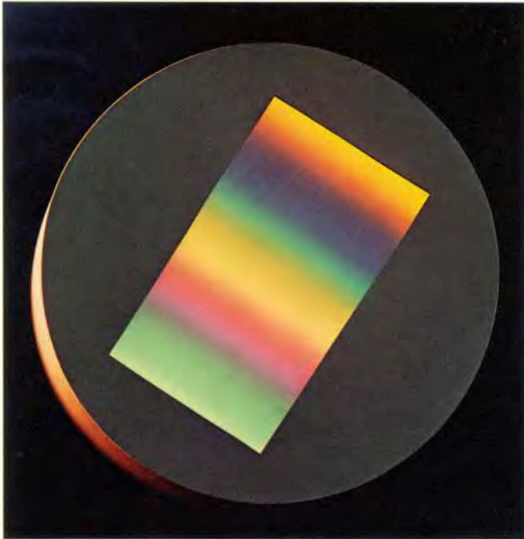
FIG. 559— Rainbow effect demonstrates the ability of a diffraction grating to sort out complex and close-lying wave lengths and electromagnetic radiation. Much of our understanding of the universe, from the minutest atomic nuclei to the far reaches of the universe is owing to spectrographs, the heart of which is the diffraction grating. So vital an element is the diffraction grating to experimental physics that it has been described as the "master key of science."
