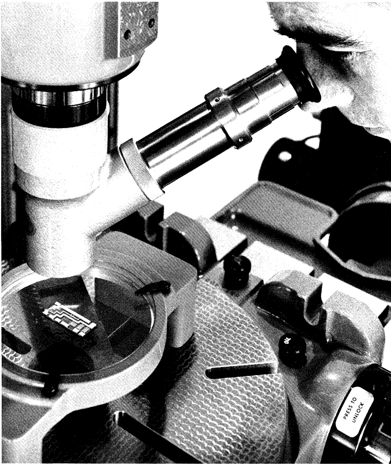
FIG. 490— Inspection of the micro-circuit component, shown mounted on the optical stage, requires use of a microscope. A collimated light source located below helps to clearly define the functional surfaces.
