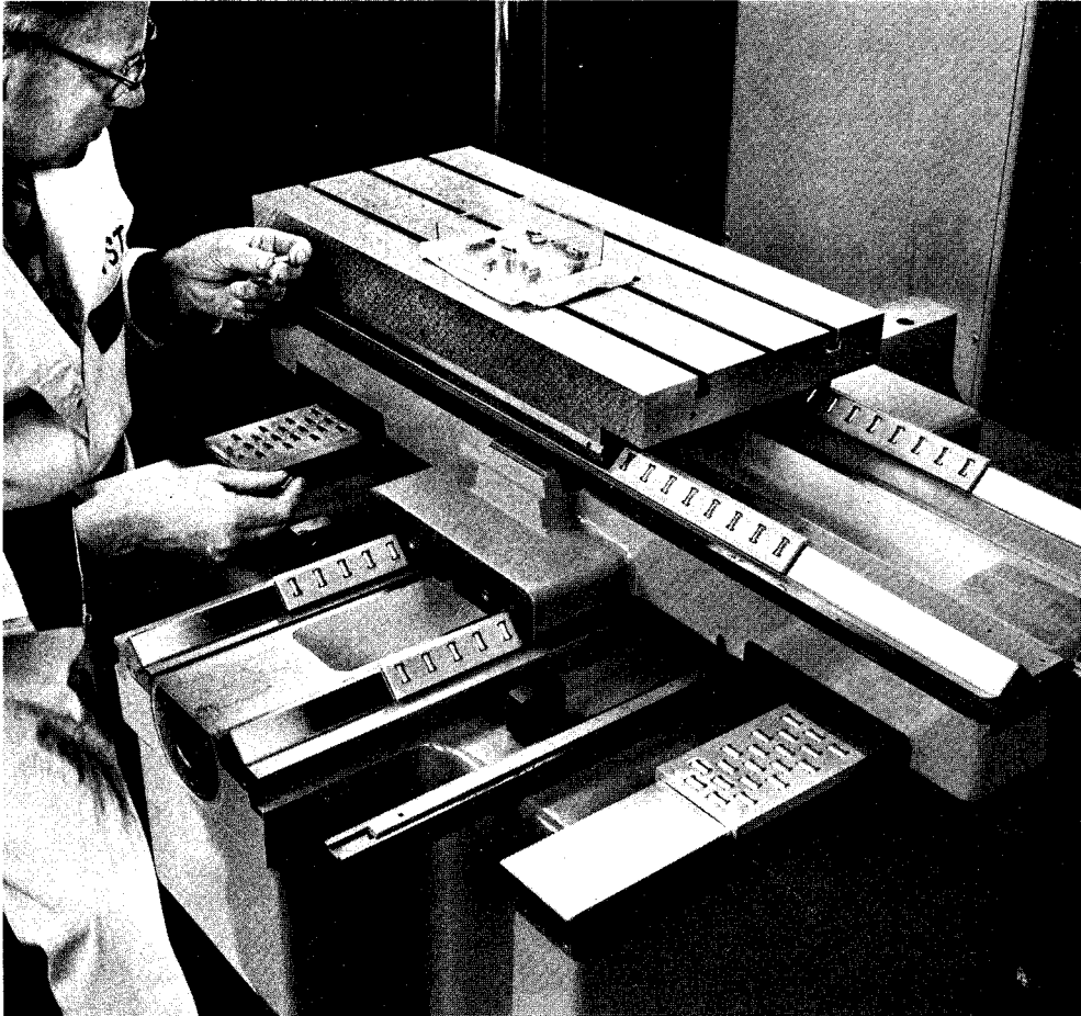
FIG. 534—A roller-way construction applied to the No. 3 base slide-ways has certain advantages for special purpose applications, notably repeatability to a fraction of a millionth of an inch [hundredth of a \mu\text{m} ]. Important applications are listed.
