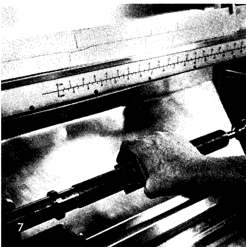
FIGS. 316 TO 324. No. 1—The thrust collar of the lead screw is lapped flat and square to the axis of lead screw. No. 2—The bearing sleeve thrust is inspected to assure flatness and squareness to the bore. No. 3—Form of the lead screw is viewed through the microscope and compared to the master 29° form. No. 4—Lines of the lead
