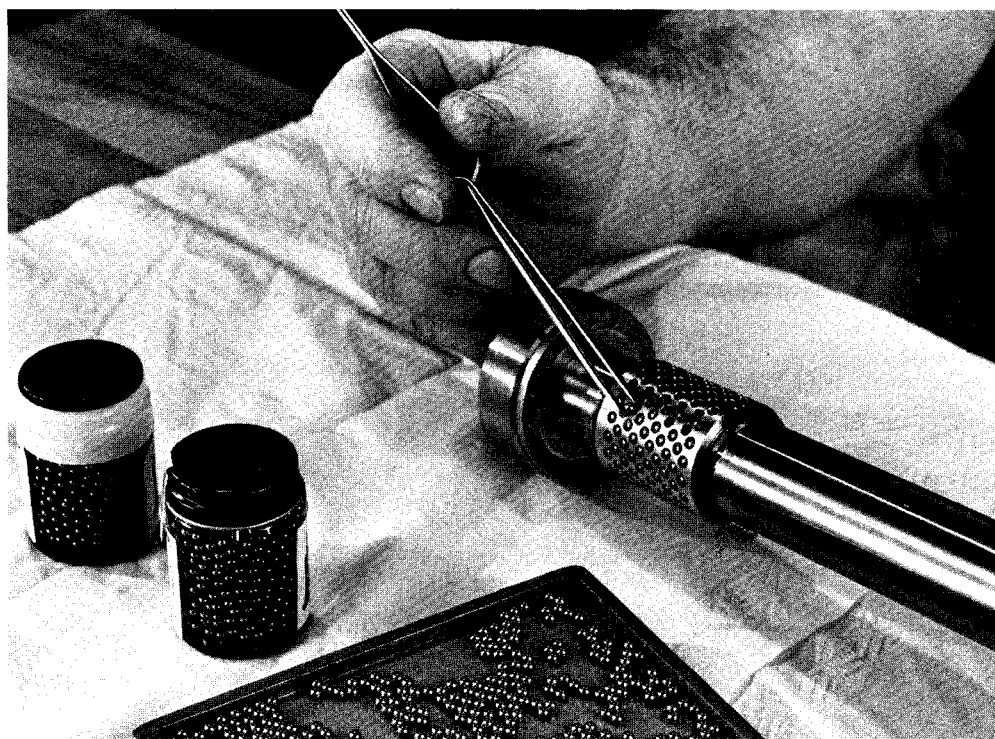
FIG. 440—Several hundred balls of identical size under an exact pre-load are used in the Universal Measuring Machine spindle. The balls are being loaded in a brass retainer.
