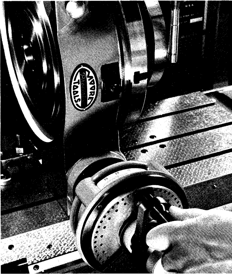
FIG. 351—The accurate worm-and-gear type rotary table is unique in that it may be used together with an index plate to divide the circle, without the necessity of
