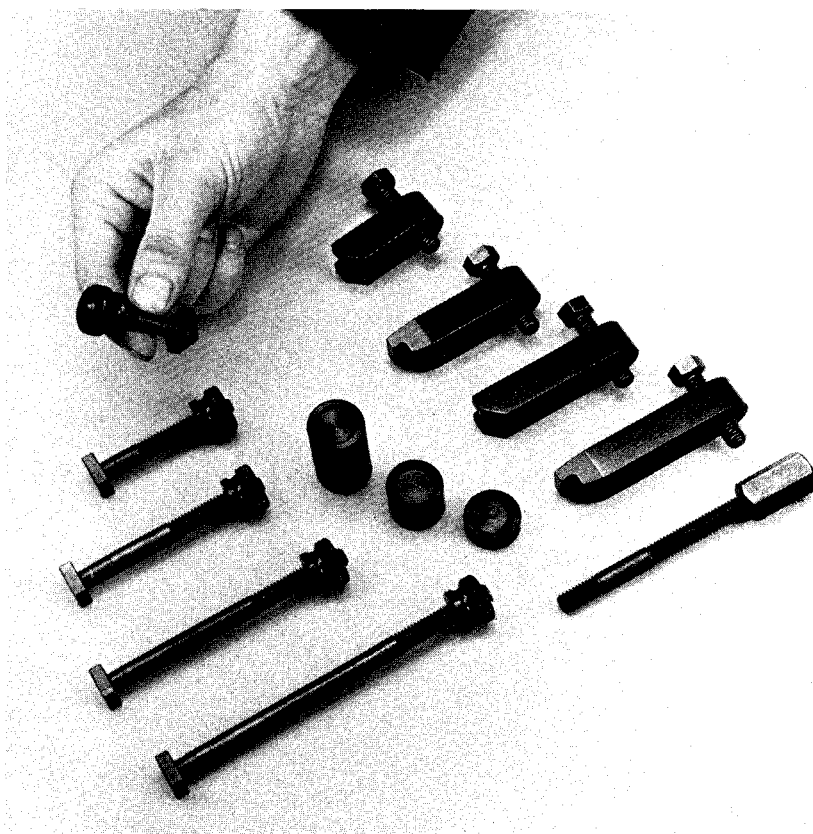
FIG. 473—A special set of workpiece clamps is furnished with the Universal Measuring Machine; a few such items are shown. An important feature of the set is the use of knurled nuts to avoid distortion of the workpiece through clamping-pressure.
