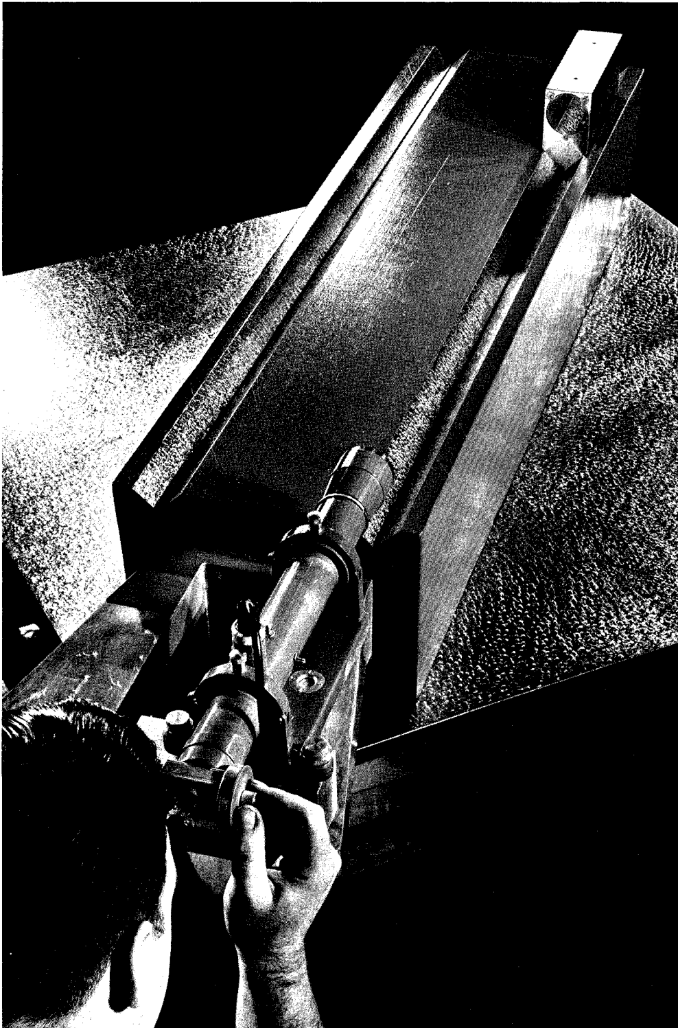
FIG. 50—The most convenient inspection for straightness in both planes is by autocollimation.
