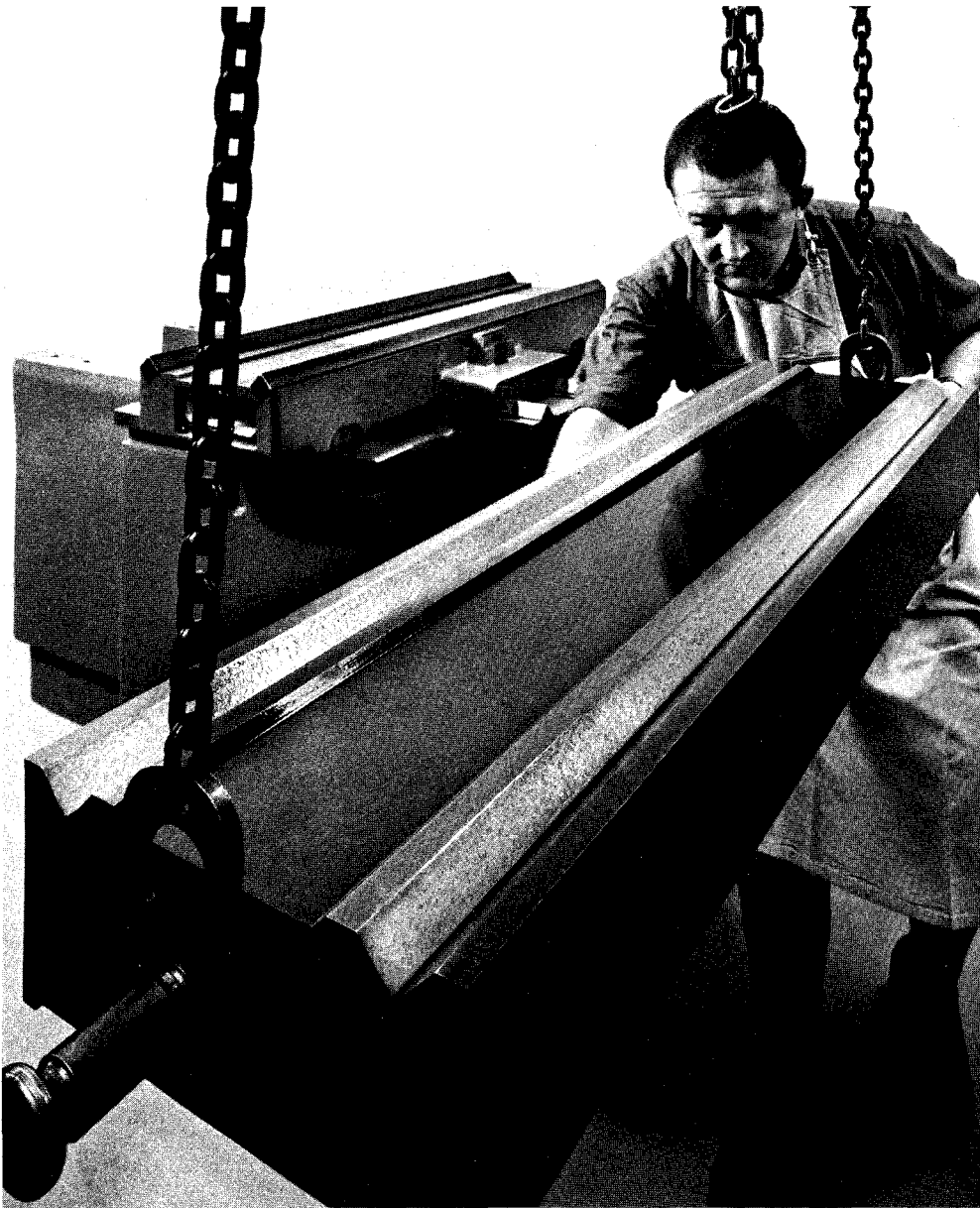
FIG. 105—The use of highly accurate checking masters greatly facilitates the lapping of the double V-way. A careful study of the bearing reveals where and how the V's must be lapped next.
