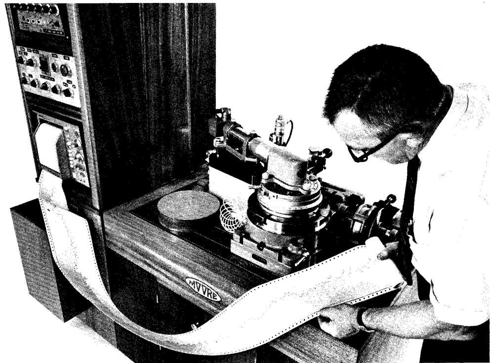
FIG. 385—The rotary table is calibrated and the error charted over one thousand, four hundred and forty positions in this automatic set-up. Time: 80 minutes. Note that worm-and-gear errors are clearly shown.
