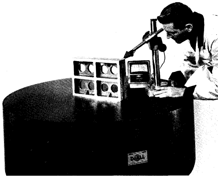
FIG. 14—The round shape of the granite surface plate is also geometrically correct for establishing flatness. Granite surface plates are the most familiar form of the flat plane and are convenient for many classes of inspection. The surface plate shown is flat to 50 millionths of an inch [0.0013 mm].
