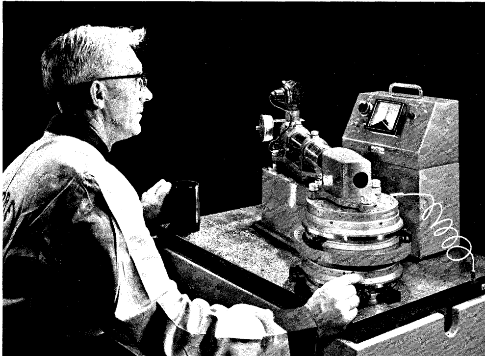
FIG. 379—Two 1440 Indexes must be employed to calibrate the 1440 Index. The classical circle-closing technique used is identical to that employed by the world's leading standards bureaus.
