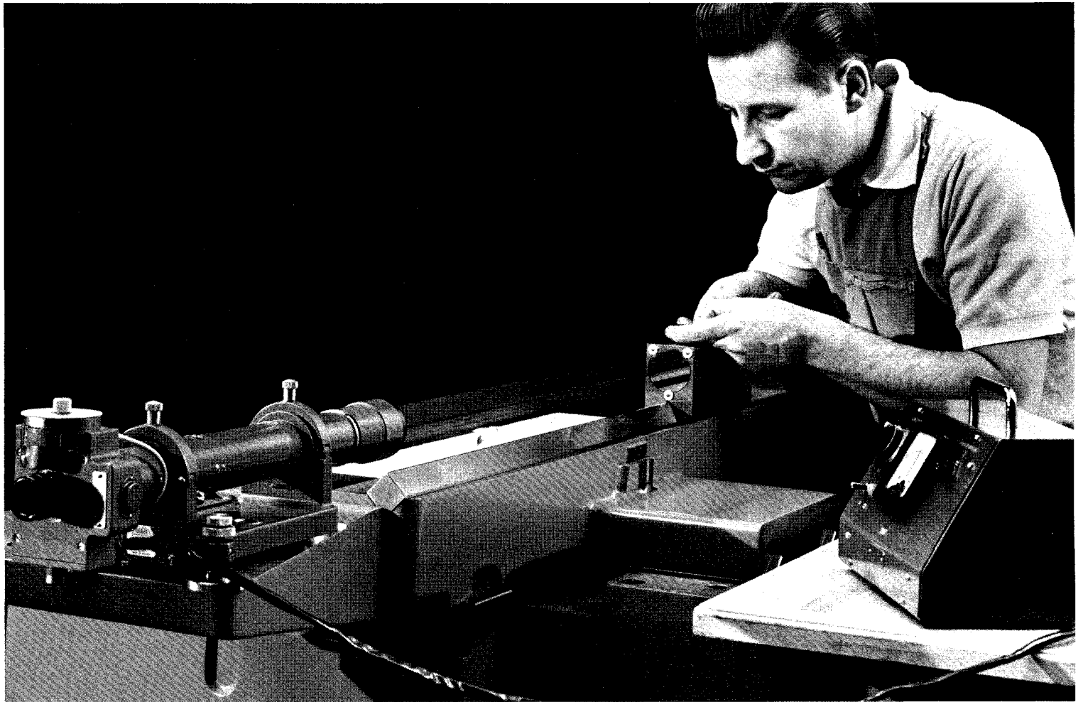
FIG. 124—The hardened and ground V-ways have now been fastened to the upper scraped female V-ways. Each V is inspected for straightness using the photo-electric autocollimator. Correction is by means of small hand laps and female double V laps.
