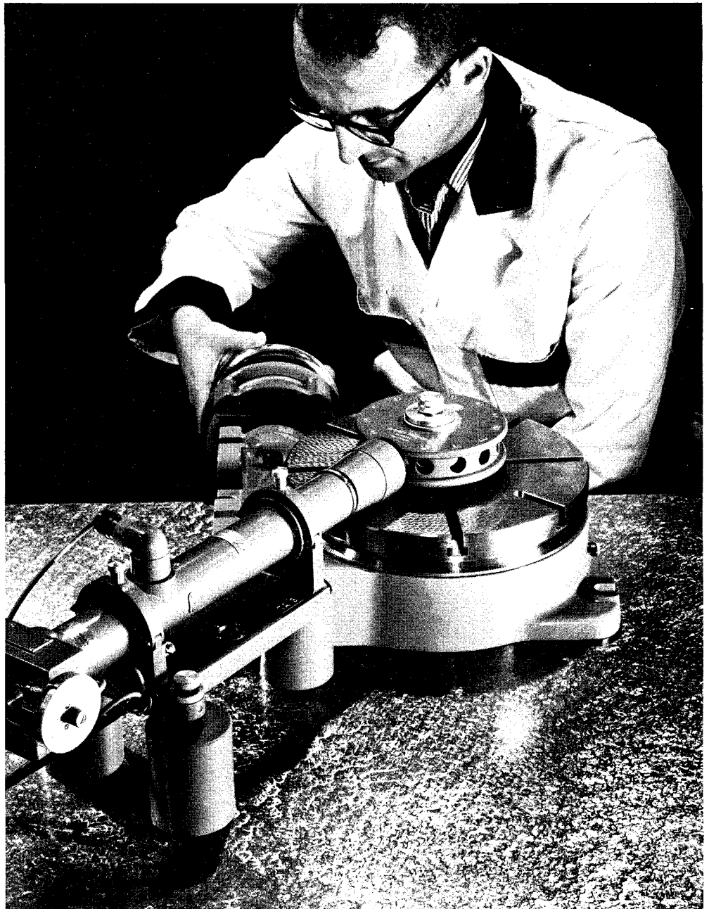
FIG. 371--Polygons were developed for calibrating circle-dividing equipment, notably rotary tables. Rotary tables are now calibrated most authoritatively by use of the 1440 Precision Index.
