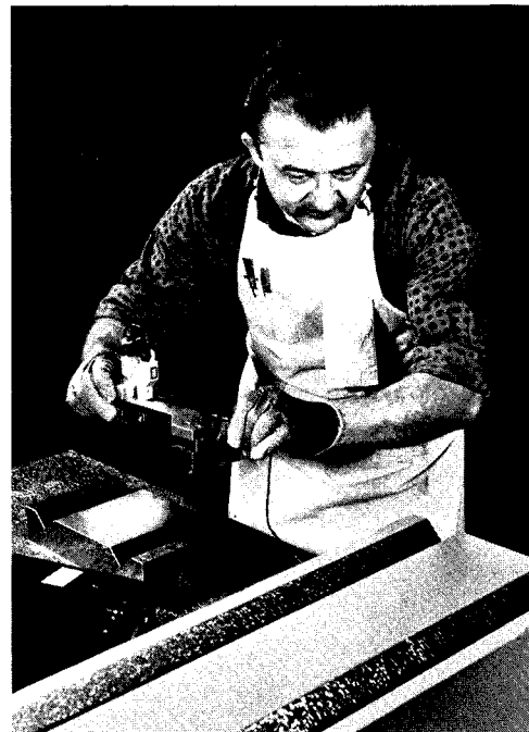
FIG. 46--Once the datum is set, the center-distance of the female double V master can be compared to the hardened master and scraped to agreement.
