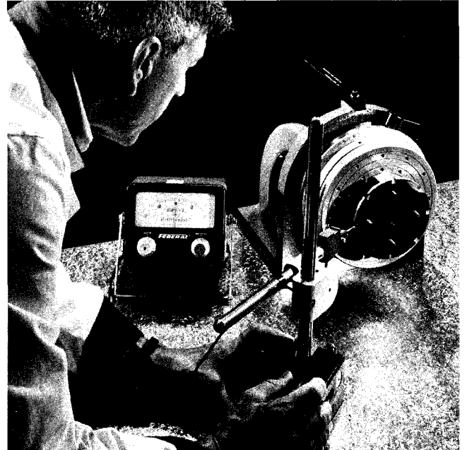
FIG. 390—The 1440 Index is mounted on a special angle iron to make possible surface plate inspection of a master notched index plate.
