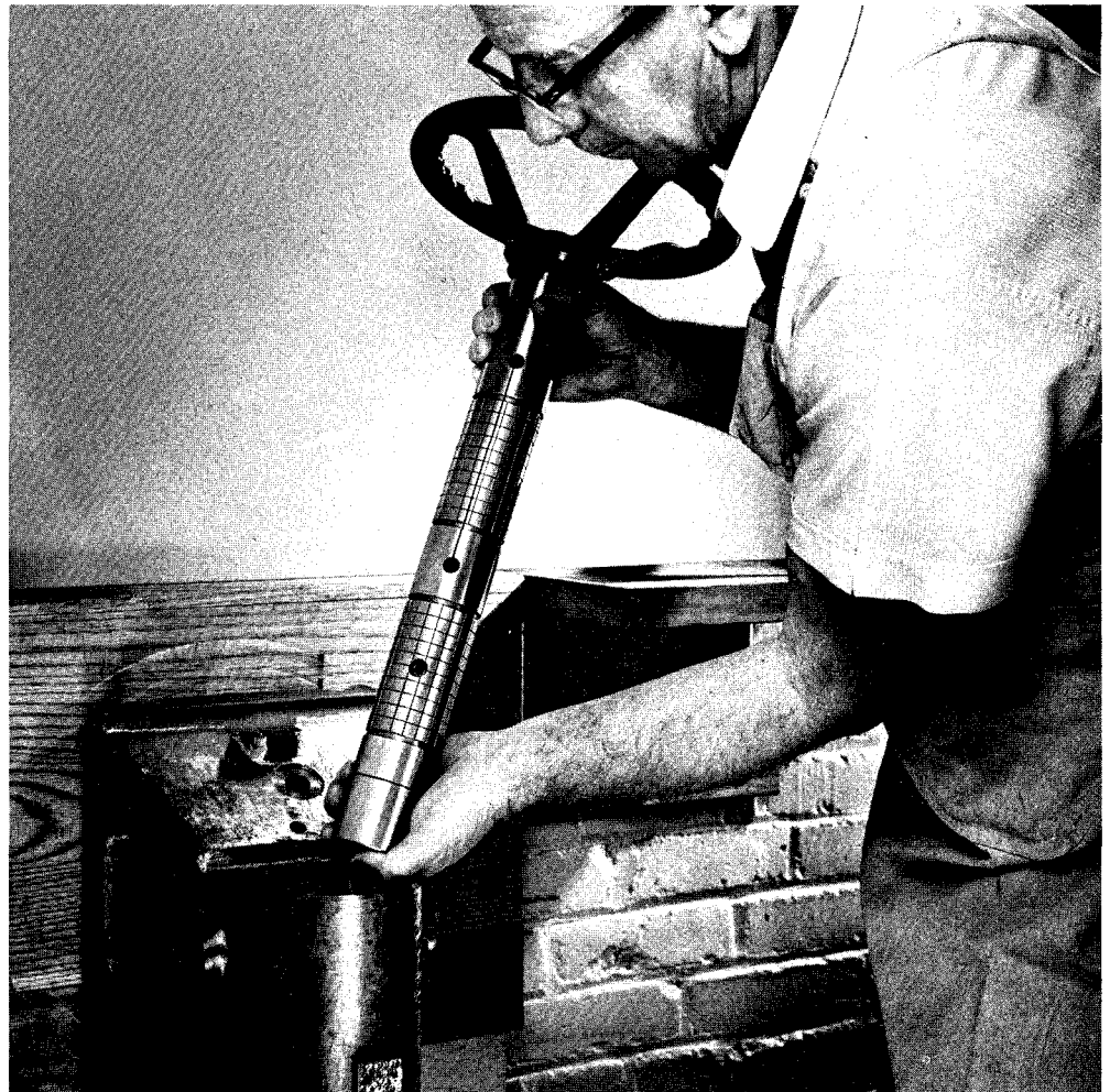
FIG. 436—Final accuracy of spindle housing elements is achieved by hand-lapping. Spindle housing is mounted vertically while its bore, consisting of two hardened and ground bushings, is lapped round, straight and to size.
