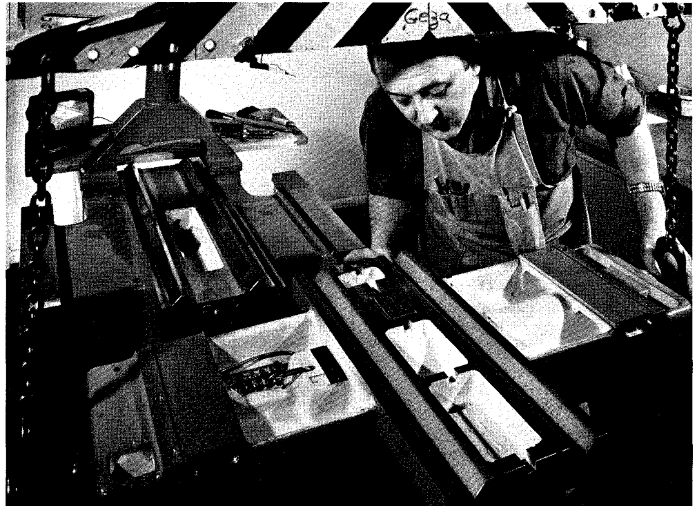
FIG. 120—Once the base flat ways and V-ways are lapped to geometric accuracy, the base becomes the “master,” and the cross-slide is scraped to match it by means of a bearing check.
