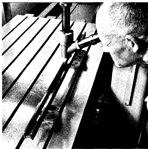
FIG. 542—The No. 5 Universal Measuring Machine has ample capacity to perform calibrations of end standards and line standards of considerable length. Shown is the inspection of a line standard using a 30\times microscope mounted in the Measuring Machine spindle.
