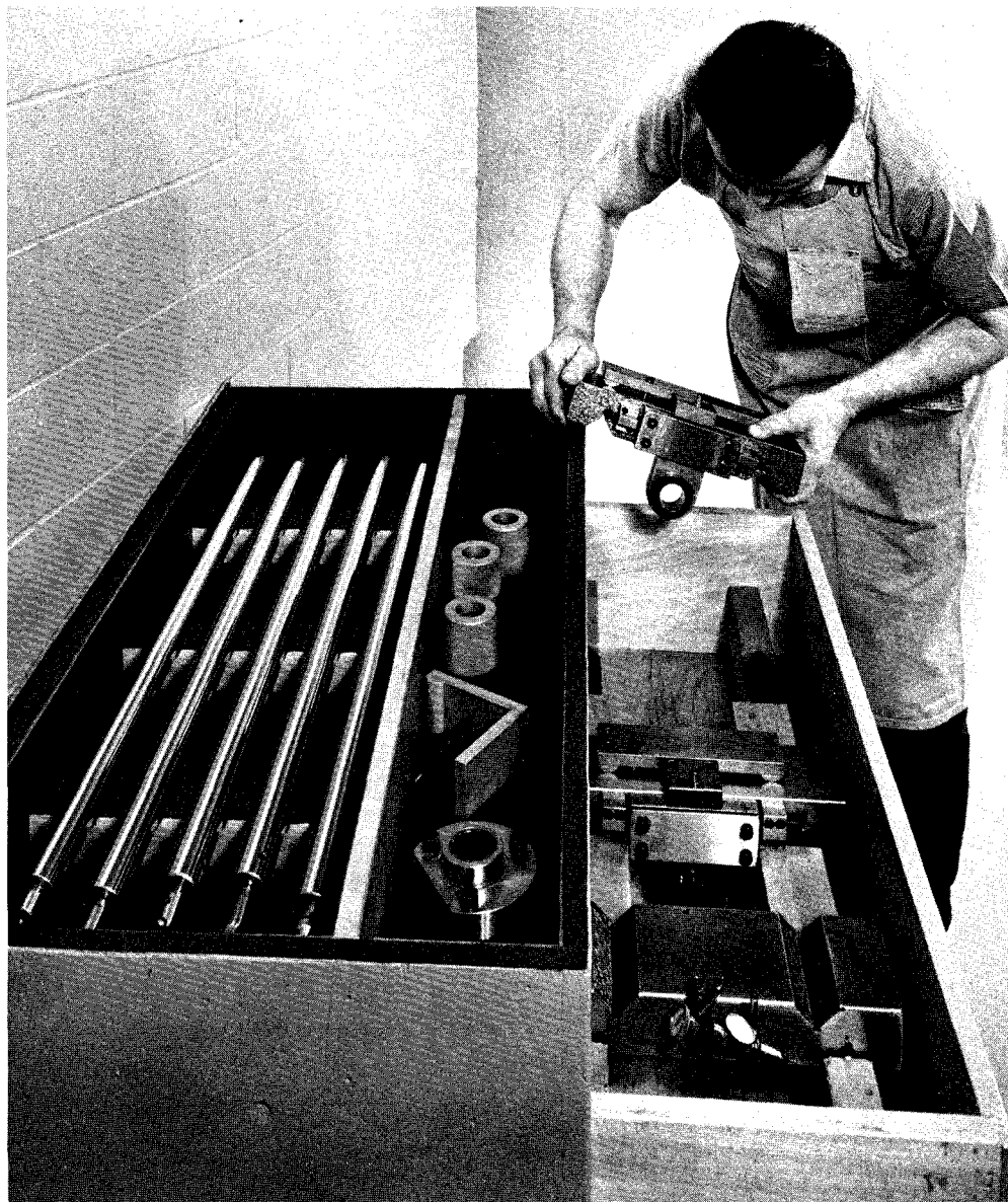
FIG. 301— Highly specialized equipment used to align the lead screw precisely in the base of the Measuring Machine.
