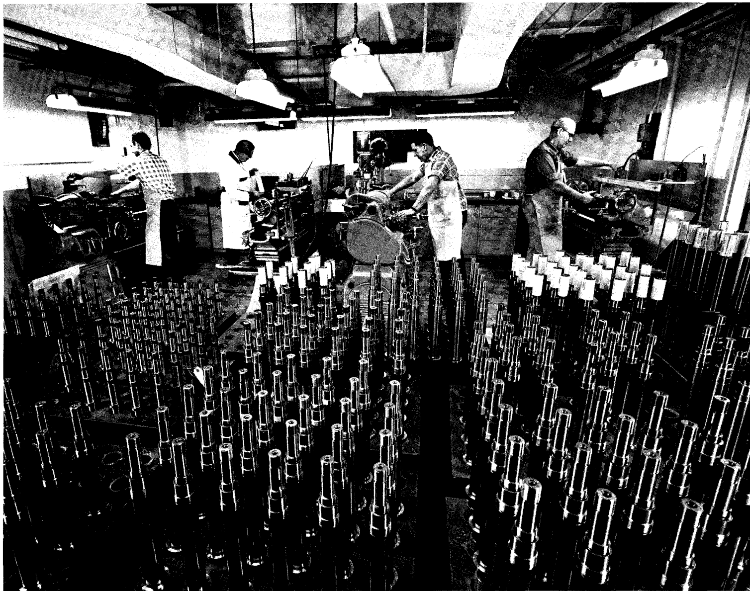
FIG. 300—Approximately 1000 lead screws are produced at Moore each year. After lead is corrected, the nut is filled and remains with the lead screw (far right), later to be part of the lead screw assembly.
