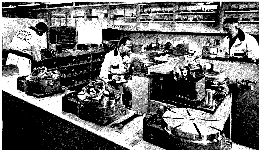
FIG. 276—Adjoining the Standards Room is the rotary table lapping and calibration area.
