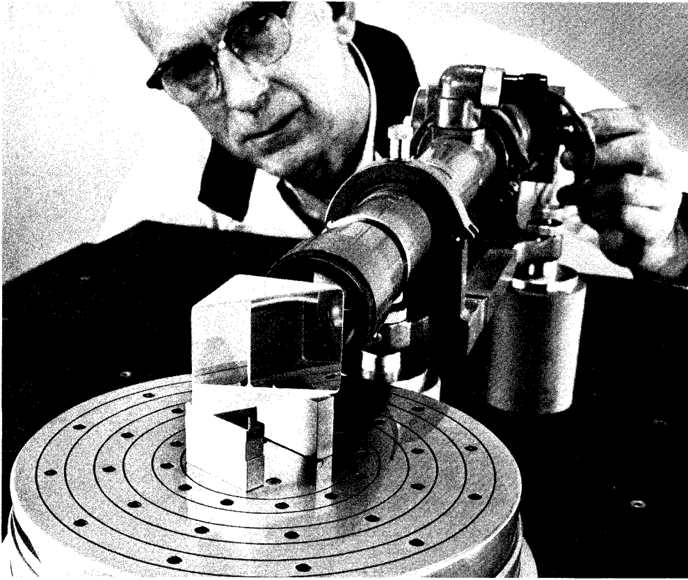
FIG. 404—Optical prisms of any angle are ideally inspected with the 1440 Small Angle Divider.
