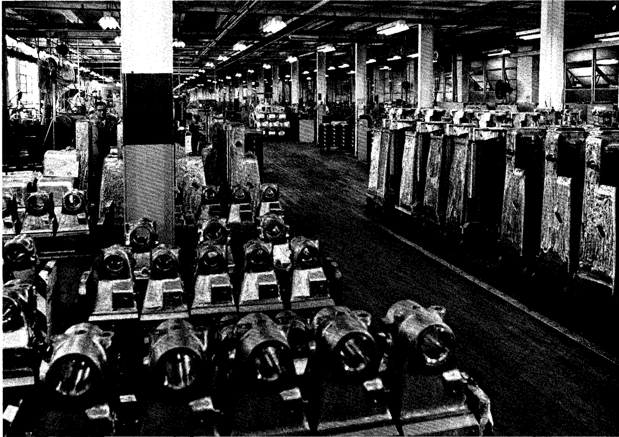
FIG. 2—The conclusion that cast iron is inherently stable is based partly on strong statistical evidence—that of thousands of castings machined and scraped to a higher order of accuracy as well as careful records kept over many decades.
