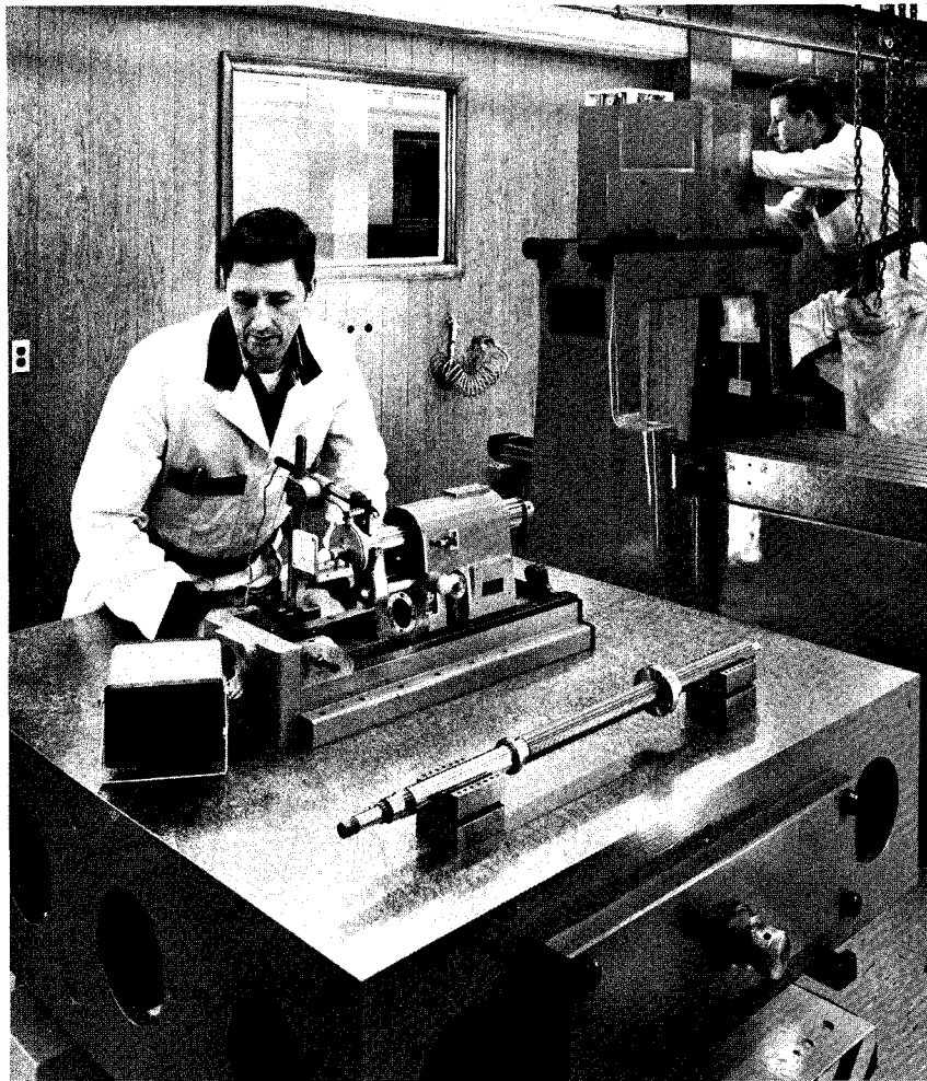
FIG. 541—The 48 inch [1219 mm] box-type surface plate, used as a master, is also convenient as a datum to inspect heavy machine parts and assemblies. Shown is the inspection of a Z axis assembly of the No. 4Z Universal Measuring Machine (background).
