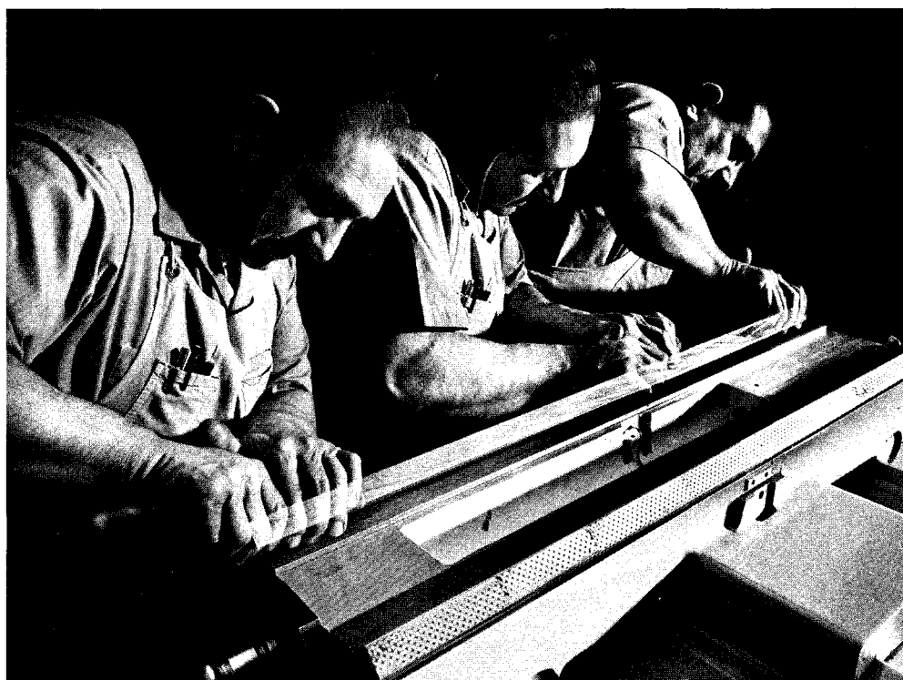
FIG. 104—Hand-lapping of the hardened double V requires an experienced hand and a thorough understanding of the geometry involved. If the surface is lapped too deep locally, many additional hours may be spent bringing the total surface down to this low point.
