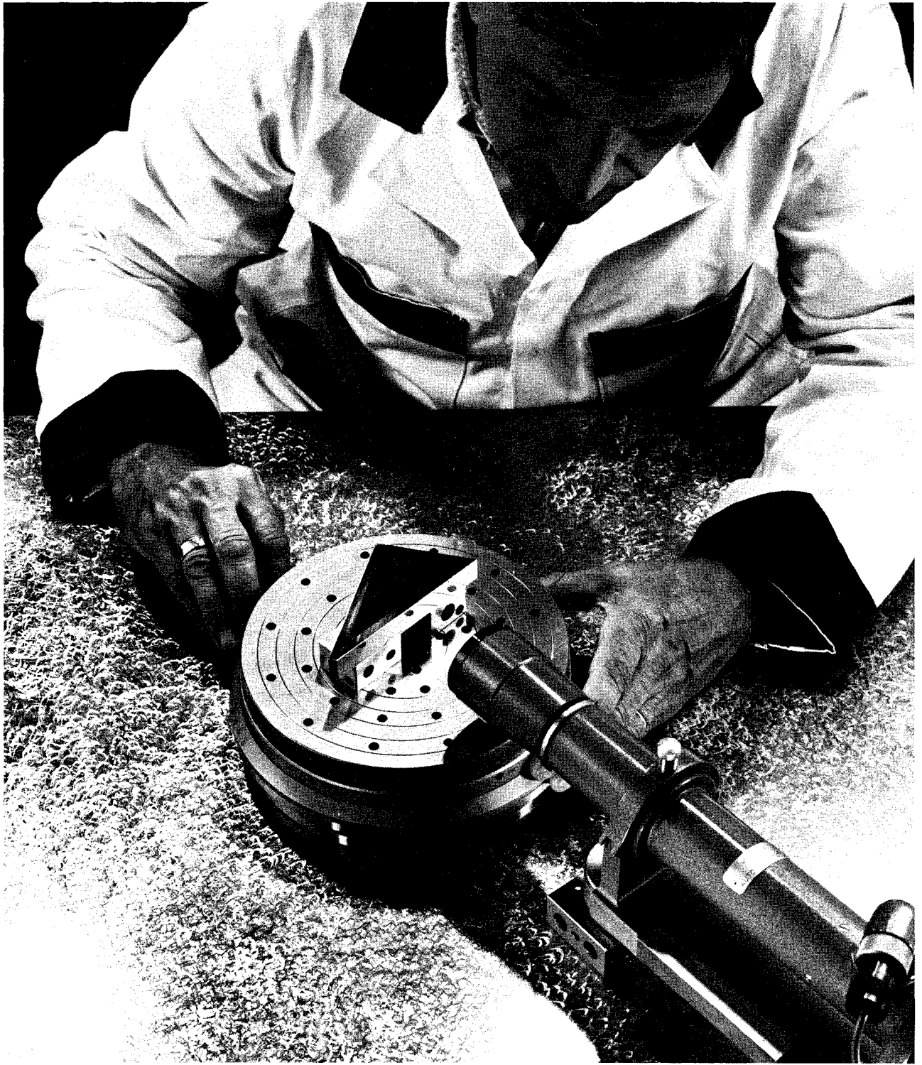
FIG. 389— The 1440 Index inspects the 30° included angle of an angle gage block, using the lapped, flat surfaces of the gage itself as reflectors.
