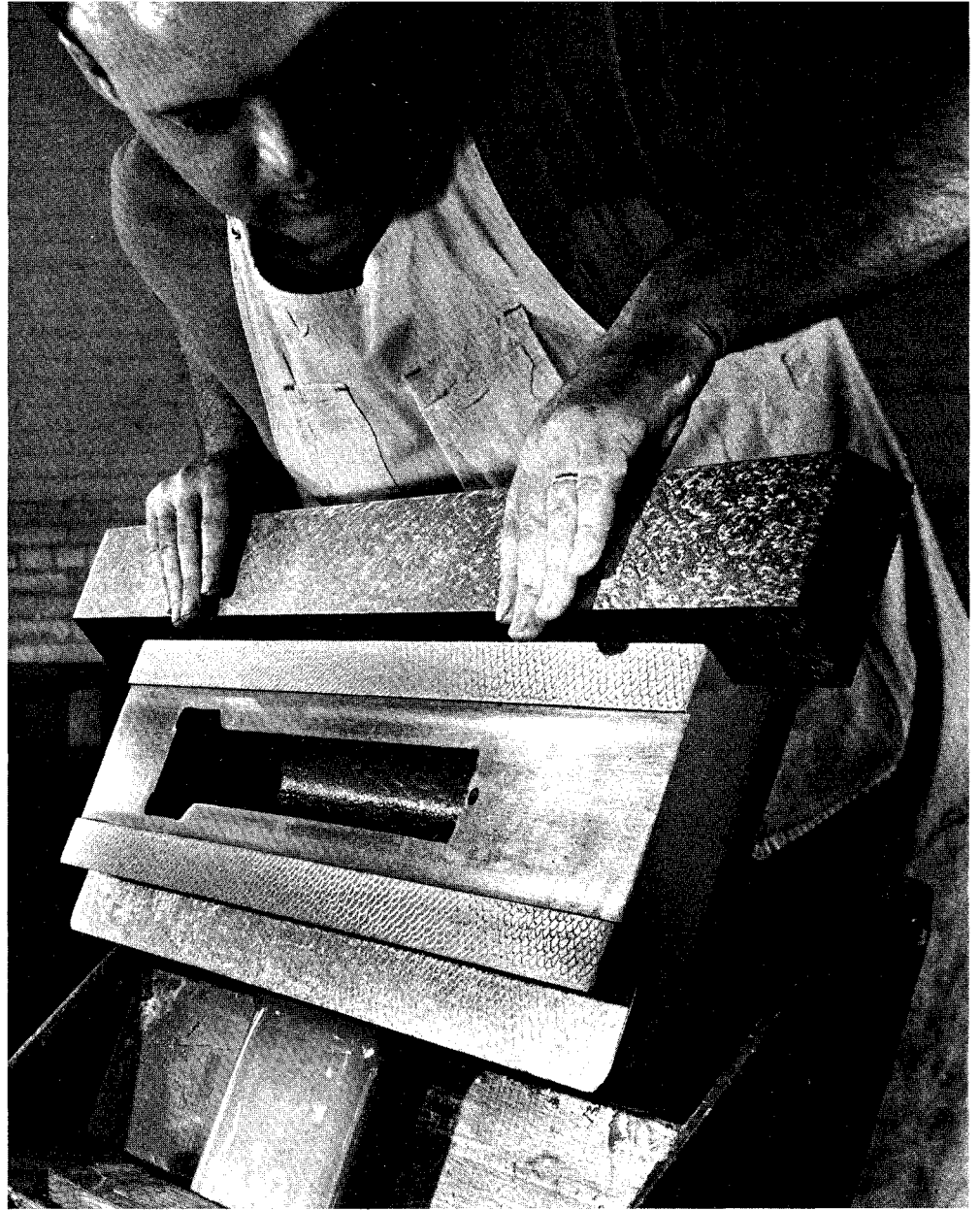
FIG. 27—A straightedge of the form shown was used to scrape the dovetail ways of No. 1 and No. 2 Model Jig Borers. Its accuracy was limited due to lack of rigidity and because its 45° form was not self-proving.
