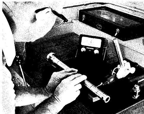
FIG. 438—Following a lapping operation, size and taper of the spindle shaft are inspected using an electronic indicator and stand.
