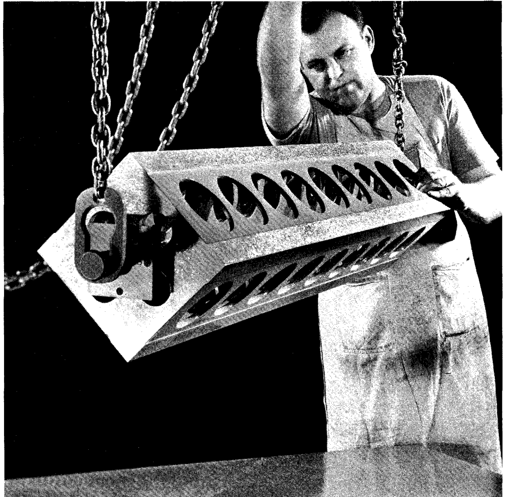
FIG. 29—The box straightedge is the best design. It is extremely rigid, its 90° form is self-proving and it is relatively insensitive to temperature change.
