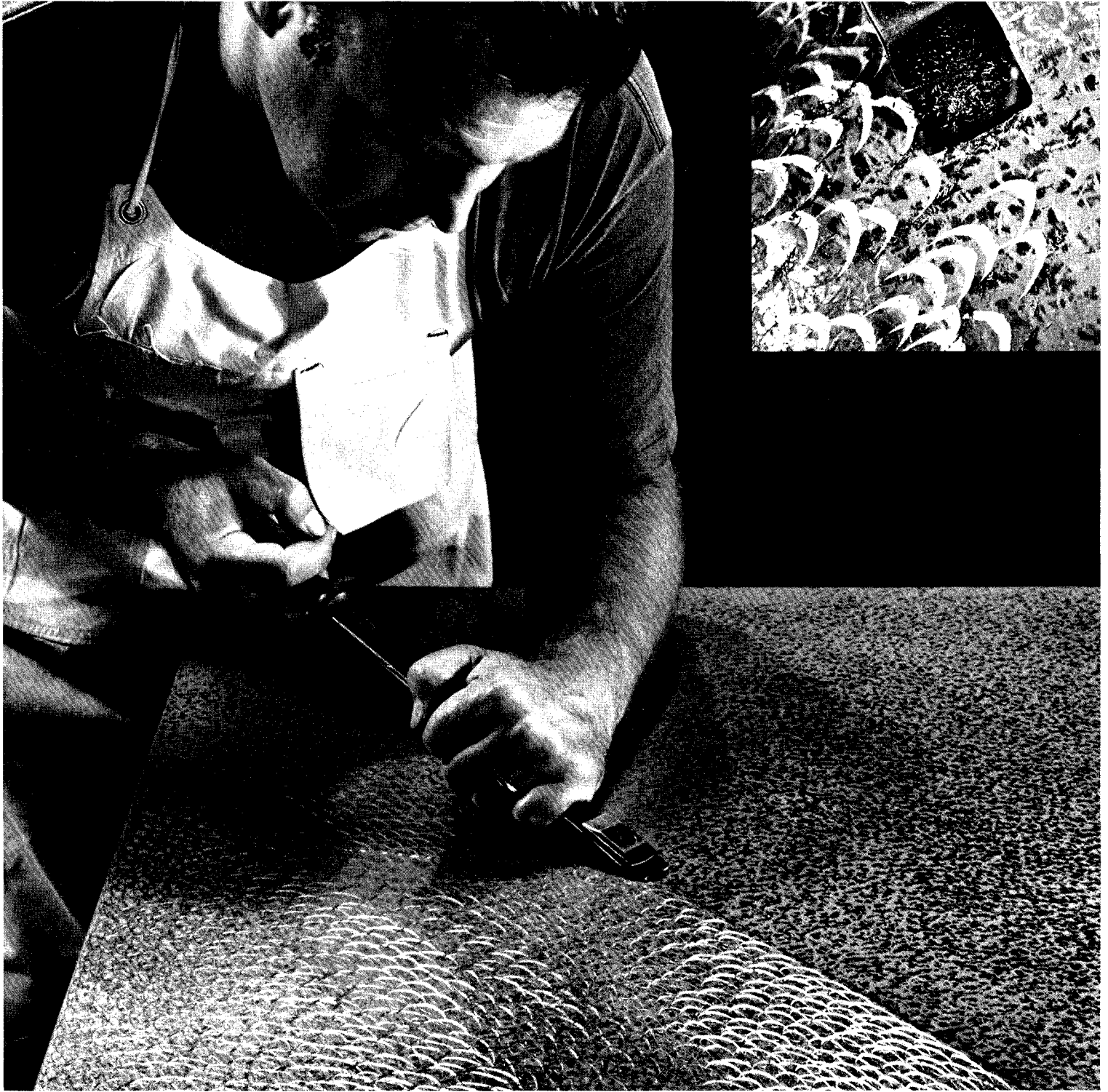
FIG. 17—A skilled, patient scraping hand can achieve almost unbelievably accurate surfaces purely by scraping to the bearing imparted, and without the use of auxiliary inspection equipment.
