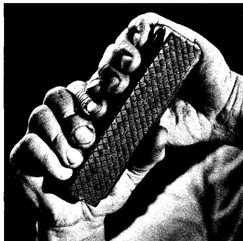
FIG. 103—Because the master laps will bend overall, small hand laps are also necessary.
