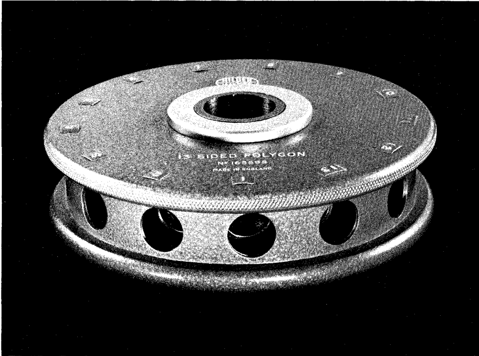
FIG. 370—The polygon is a principal circle-dividing standard, having a number of reflective surfaces on its periphery set to a specified angle for use in conjunction with an autocollimator.
