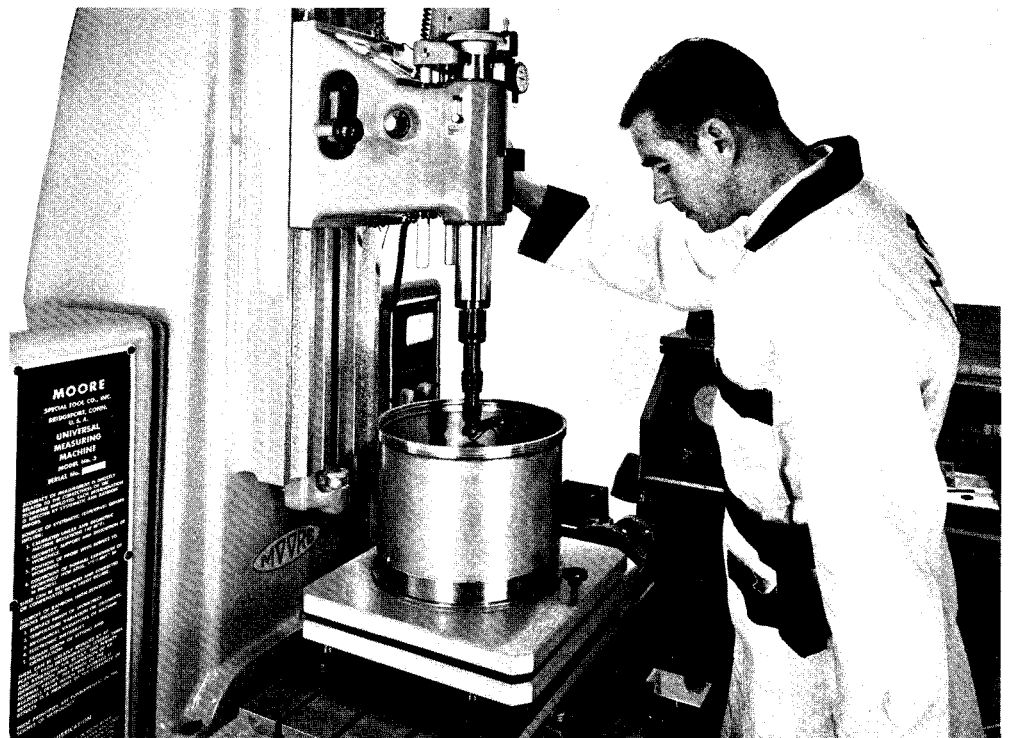
FIG. 442—An accurate spindle housing travel at times proves convenient when the piece to be measured requires a range of vertical adjustment beyond that of the quill alone, such as with this large stainless steel part.
