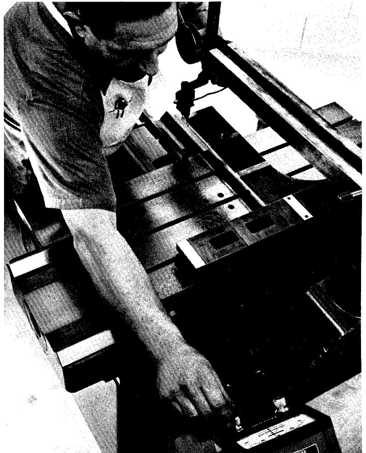
FIG. 135—Final inspection of squareness employs a nitralloy T-square, accurate to 10 millionths of an inch (0.00025 mm). The square is self-checked by reversal. Tolerance of squareness of the machine axes is 20 millionths of an inch (0.0005 mm).
