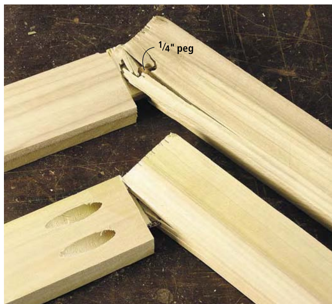
The 54 lb. anvil also damaged both joints. Note how the peg in the tenon and the screw destroyed the edge of the stile.
