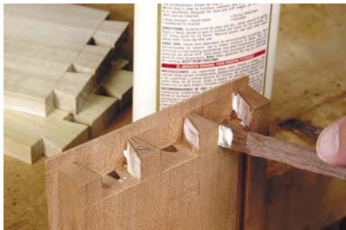
I apply glue only to the long-grain surfaces of the pin boards. Glue on the tails will only squeeze out and make a mess.
