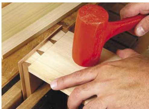
A gentle tap with a dead blow mallet completes the assembly of the joint.
