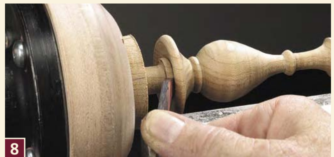
5 Here I have mounted the second half, cut a recess to fit the first half, and hollowed out the interior.
