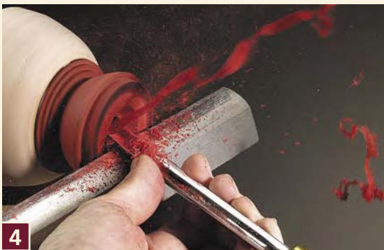
2 Mount the first half of the globe stock. Cut a straight shoulder on the end, and rough in the shape of the ball.
