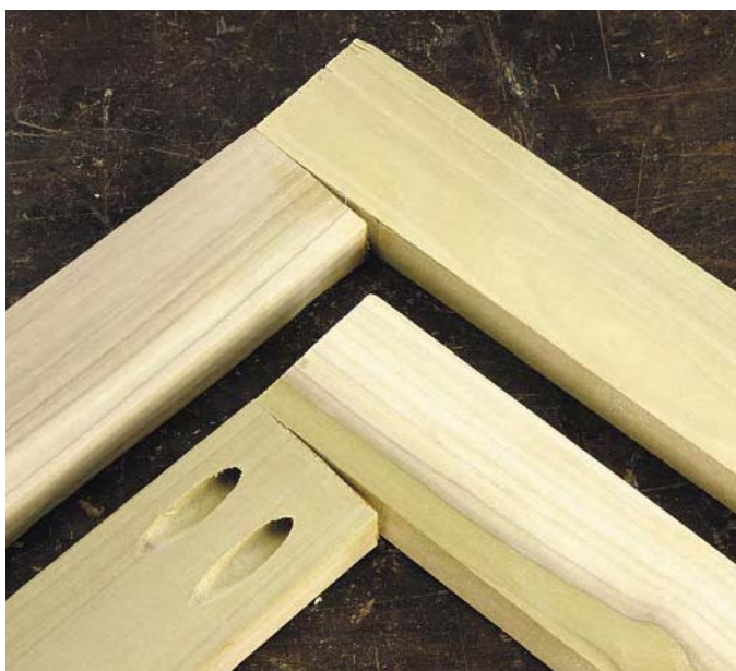
Mortise-and-tenon joints and pocket-screwed butt joints showed similar amounts of damage from the 26 lb. anvil.
