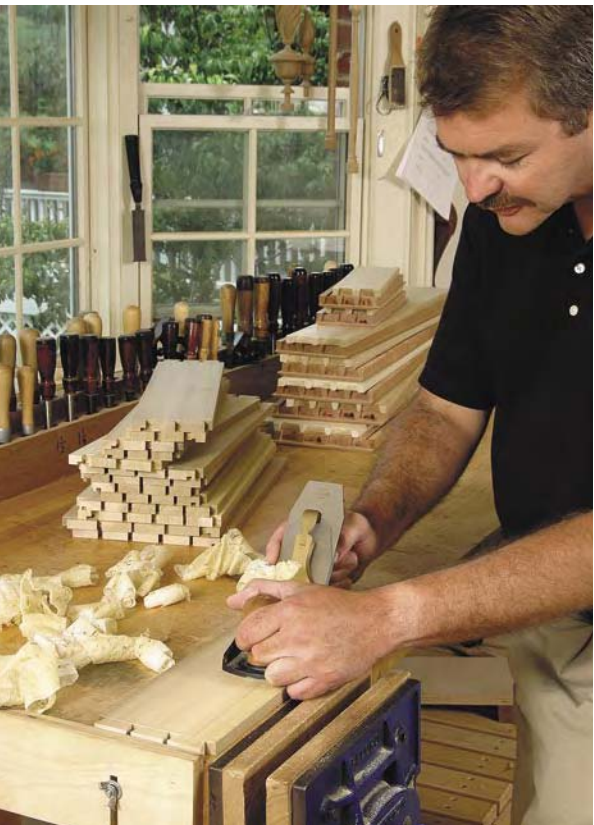
I use a smoothing plane to smooth the inside of the tail boards before assembling the drawers. The inside of the pin boards are done before layout of the joints.
