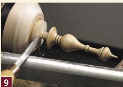
7 Mount and turn the long (lower) spindle. This is just like turning the icicle ornament; see those instructions for more detail.
