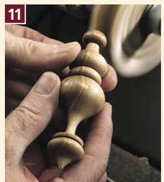
8 Make a wide, undercut flange and a 1/2" -diameter tenon at one end.
