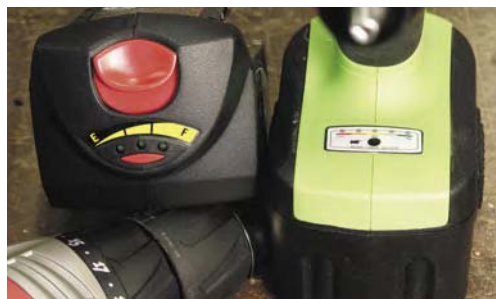
Skil and Moty-Ko offer fuel gauges to help you determine how much juice is left in a battery. A nice idea, but we're not sure how accurate or useful these gauges are.
