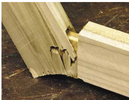
Not much material was left between the mortise and the edge of the wood in the thinner material.
