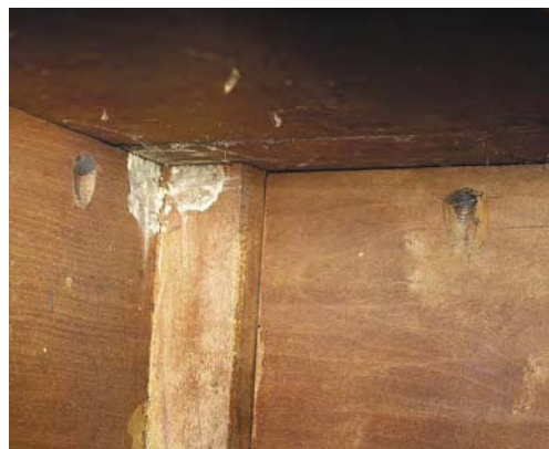
Pocket screws, like these crudely formed examples, were often used by Shaker craftsmen to hold tops in place.
