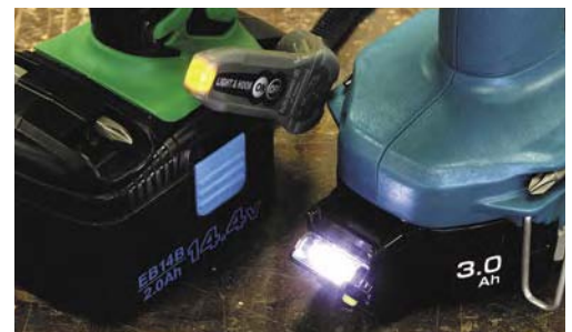
The Hitachi and Makita drills have multi-position LED lights. Both are handy in a dark corner, but neither are a reason to choose these drills over others in the test.
