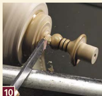
7 Mount and turn the long (lower) spindle. This is just like turning the icicle ornament; see those instructions for more detail.
