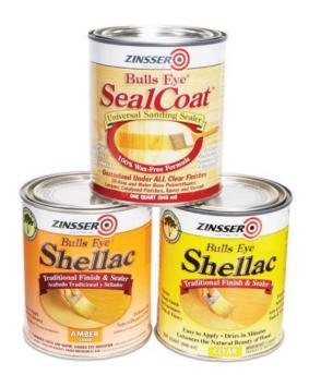
Zinsser's "Amber" shellac is a ready to use orange shellac and their "Clear" shellac is a blond shellac. Both of these products contain wax and are mixed to a 3- pound cut that should be thinned to a 1-2 pound cut before use. "SealCoat is a 2-pound cut of dewaxed blonde shellac. SealCoat is a universal sealer that adds just the right amount of warmth and color underneath a
