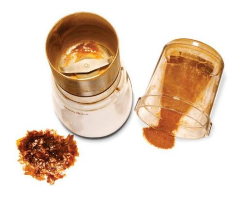
Shellac flakes take quite a while to dissolve. When my shop is cool, I've had to wait more than 2-days. Too often I have failed to plan ahead and been forced to wait for my shellac to dissolve before work could progress. You can greatly reduce the time it takes to mix shellac by grinding up the flakes. A simple blade-type coffee grinder does the trick.
