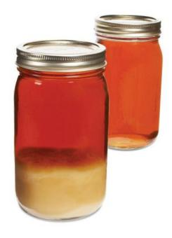
Should you buy waxed or de-waxed shellac? Wax occurs naturally in shellac. If shellac is going to be the only finish, then shellac with wax works fine. The wax decreases drag when padding or brushing on shellac. If shellac is used as a sealer or undercoat for other finishes, choose the dewaxed version to avoid adhesion problems, especially with polyurethane. Dewaxed shellac
