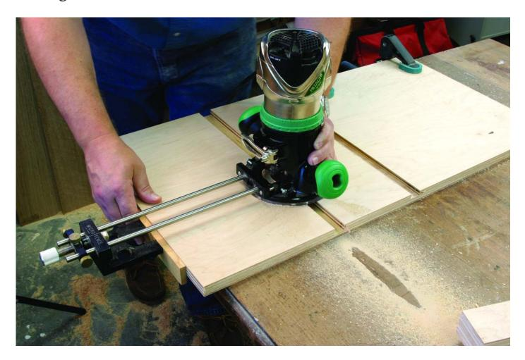
After making my centered  $3/4" \times 3/8"$ -deep dado, I cut both the side  $1" \times 1/2"$ -deep dados using two passes with the same bit.
