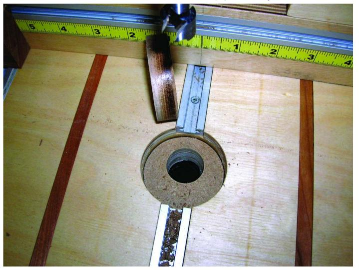
The two-plug system brings the insert flush to the table surface. Also notice the offset location (the through hole is where the bit will drill) to keep the discs from spinning.
