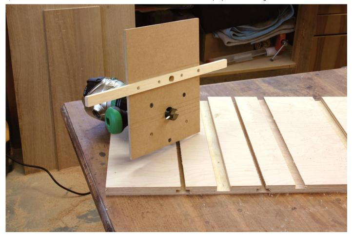
My jig to guide the T-slot cutter is simply an auxiliary base plate for the router and a 3/4" x 3/8" strip to guide in the 1" slots.
