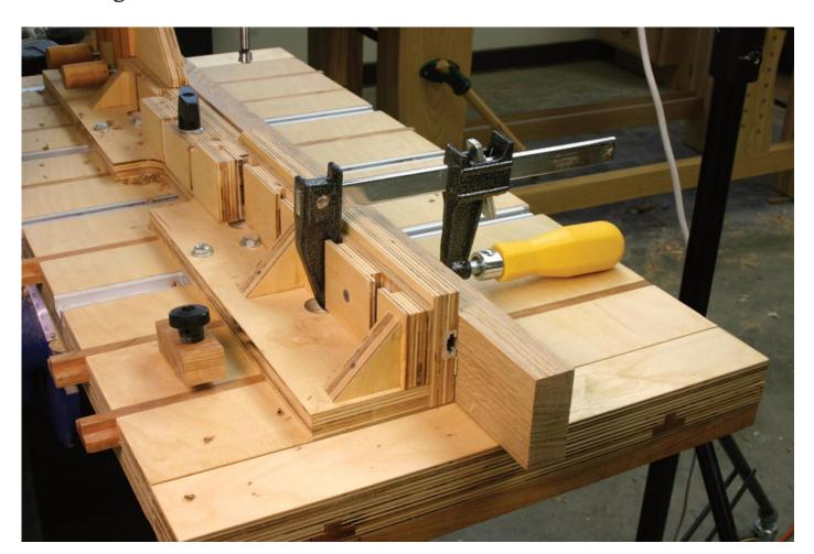
The fence can be simplified to the basic base, front and triangular braces, but I added the T-slotted rear fence to make it easy to attach a clamp to the fence. The T-slot lets the head of the F-style clamp slide into place, and holds it there.
