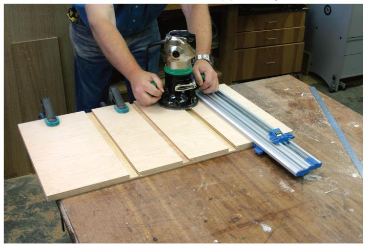
The second 1" dado must be parallel to the first, so if you use a router guide as shown here, measure carefully from the first dado to align the cut.
