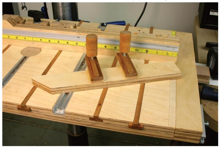
For working with taller objects, a taller fence (part K) is handy. By utilizing the T-slots in the rear fence, I easily adapted an auxiliary fence to slip into place on the right or left side of the table.
