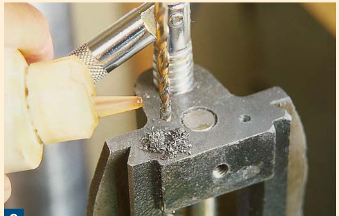
8 Using a #7 drill bit for a 1/4"-20 tap, drill the two holes. Use some cutting oil to keep things cool.
