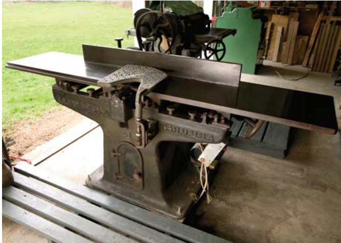
This Fay & Egan 16" jointer from 1912 is the machine that started Batory on his road to self-discovery and historical conquest.
