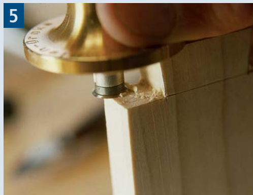
5 The Tite-Mark gauge can be used like a chisel to remove waste from between the tails and on the ends of the joints, as shown. If you sharpen the tool's flat cutter, it will slice wood like a chisel.
