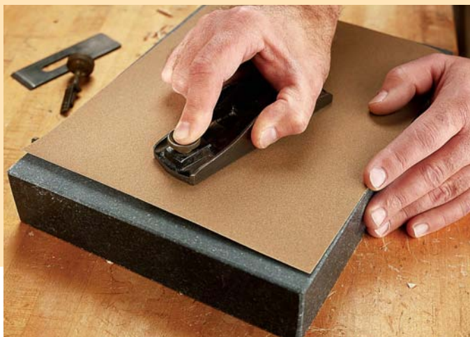
The sole of a block plane can be trued on sandpaper (#100 to #320 grit) supported on a granite reference plate.
