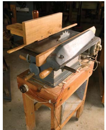
The Craftsman tilt-top table saw was revolutionary for the early '40s. All of today's table saws owe their lineage to this machine. We now tilt the arbor rather than the table, but it's nice to see the beginnings of such an important machine.
