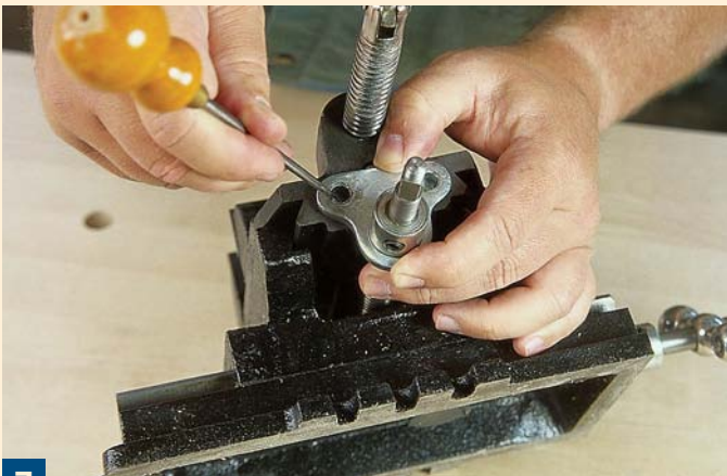
7 There are no tapped holes on this side. Turn the vise on its side and carefully mark two holes on the vise. An awl leaves an easily identifiable mark.
