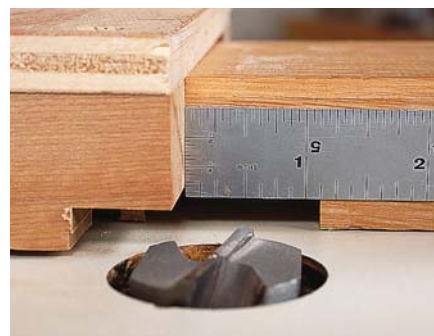
Position the stop by measuring from the shoulder of the cut in the sled's fence. Use the same bit for tenoning so the shoulder cut remains accurate for setups and for backing up the tenon shoulders.
