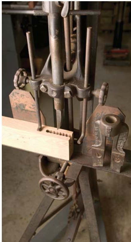
While still very functional, this foot-powered mortiser/tenoner (purchased for $35) is a lot more fun as a conversation piece.
