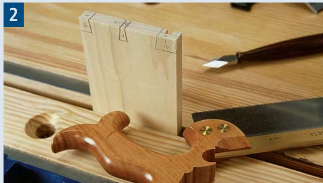
2 Mark out your tails on the end grain and the outside face of the drawer side. Strike your lines with a marking knife followed by a mechanical pencil. This will increase your accuracy. Mark the waste portions of the joint with an "X" and then make your cuts.
