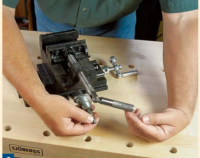
6 Slide the vise out of the dovetailed ways and spin the vise 180°. Rethread the rod into the center guide block from the opposite side.
