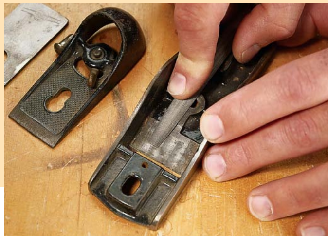
A small mill file can rescue the bed of an inexpensive plane by ridding it of any defects. However, a light touch is key.
