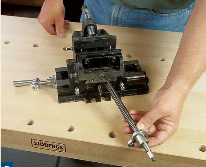
5 By turning the threaded rod counterclockwise, you can unscrew it from the center guide block and pull it free of the vise.
