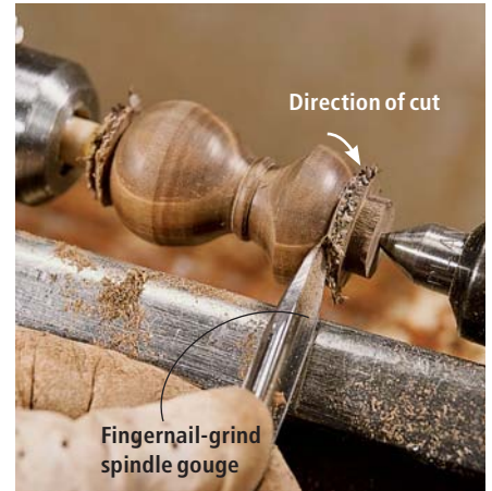
Refine the shape and make the finishing cuts with a long-fingernail-grind spindle gouge.
