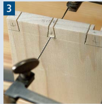
3 Remove the waste between the tails with a fretsaw or coping saw. The closer to the bottom of the tail you get, the less clean-up work you'll have with a chisel.
