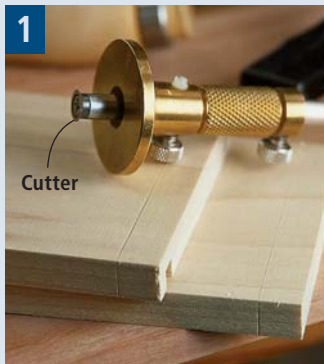
1 A sharp and high-quality cutting gauge, such as the Tite-Mark, makes lines that are easier to see than with a scratch gauge, which uses a pin.
