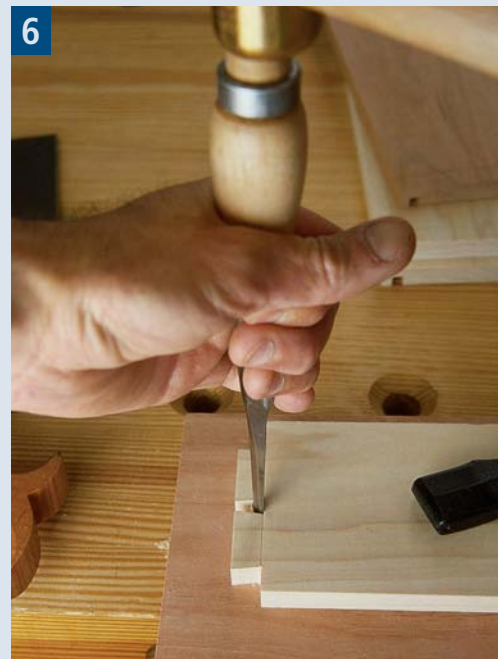
6 Remove the remainder of the waste with a bench chisel. The most important thing to note here is you should stand so you can see when the chisel is perfectly perpendicular to the work, as shown here.
