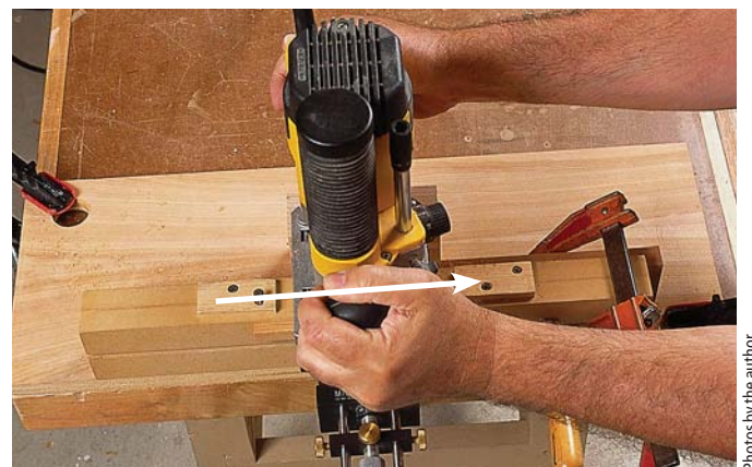
The jig provides support under each plunge post, which enables you to plunge your router smoothly. When cutting, move the router in the proper direction, so the bit's rotation pulls the edge guide against the support.
