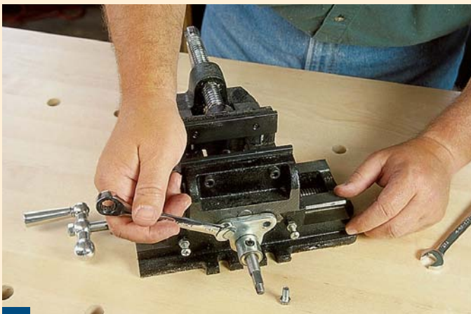
3 Then remove the two machined bolts holding the cover plate in position.
