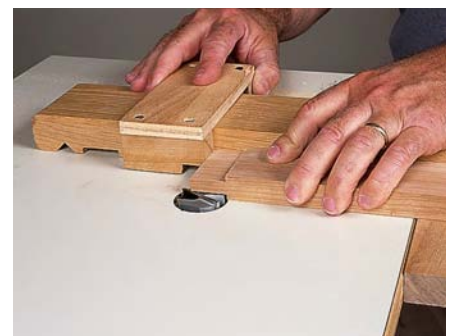
Cutting your tenon takes only one pass per cheek. Lay the work on the table, pull it against the sled's fence and stop and feed it across the bit. The bit cuts the cheek and shoulder simultaneously.
