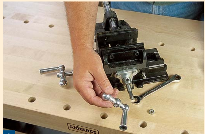
2 Remove the front handle by pulling it straight off the threaded rod.
