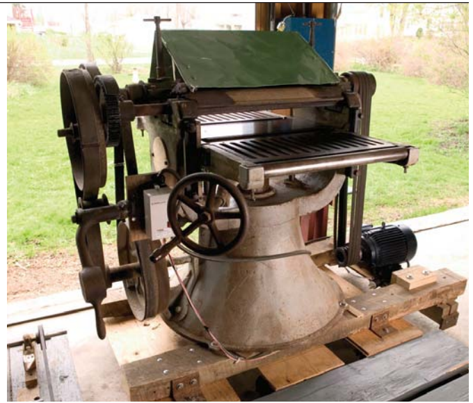
One of the most difficult tasks when rehabbing Batory's John A. White planer was finding reproduction leather pulley belts. It was a lot of work, but the belts are one of the coolest aspects of the machine.
