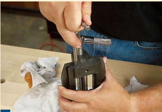
9 Using the corresponding tap, cut the threads into the two holes. Again, cutting oil makes the process smoother.
