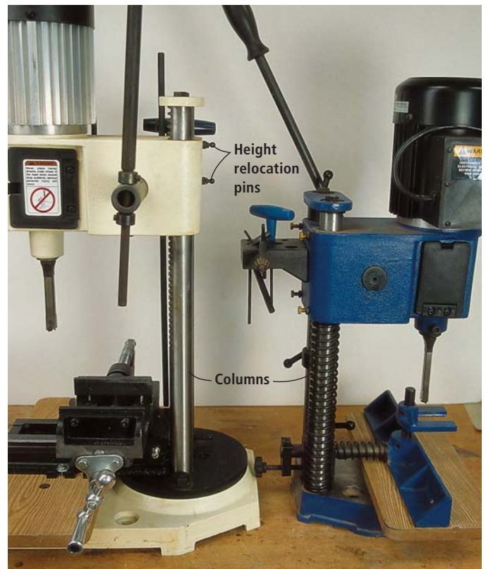
These two mortisers quickly make the height difference apparent. The Shop Fox, left, has longer columns and is capable of being adjusted to gain additional height by relocating the gas cylinder on optional pins.
