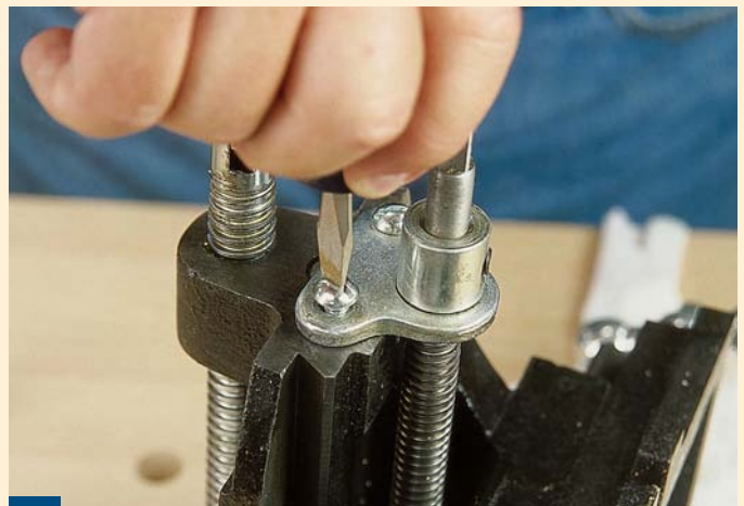
10 Last, screw the plate in its new location and your reworked vise is ready to work. PW
