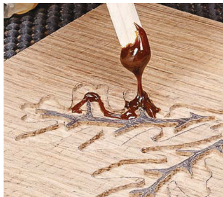
▲ Tinted epoxy anchors the inlay into the recess. You only need a small amount to prevent squeezeout.
