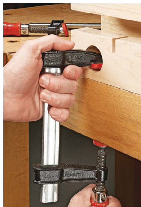
▲ A pair of openings at the front of the bench accept the head of a bar clamp to secure the bench.
