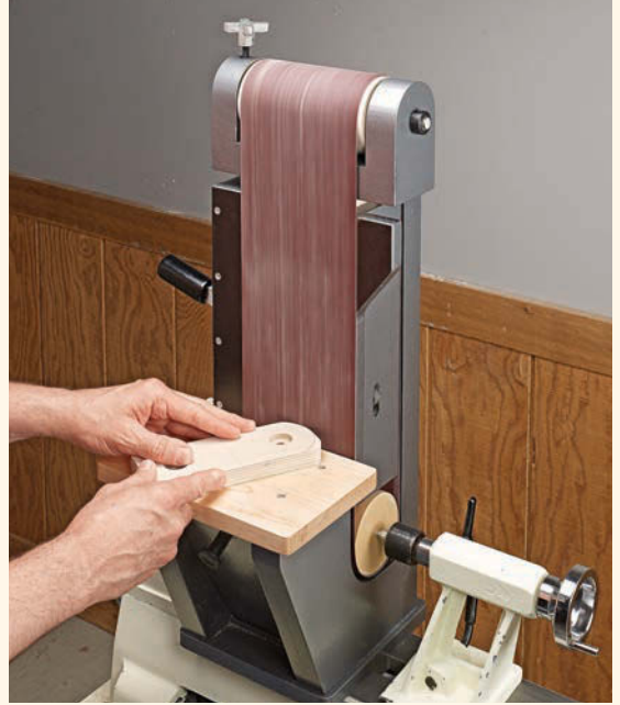
▲ Lathe Belt Sander. Get double duty out of your lathe by building this belt sander attachment. It mounts directly to the bed and is driven by the headstock of the lathe. Plans begin on page 30.
