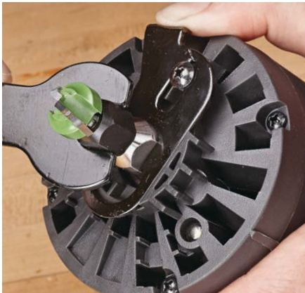
▲ A spindle lock means only one wrench is needed to change bits but the motor may need to be removed to access the lock.
