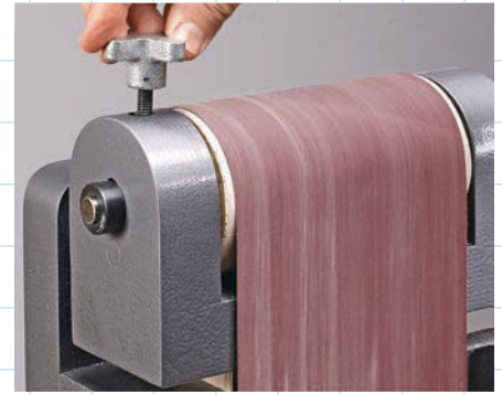
▲ A simple tracking mechanism keeps the sanding belt centered on a pair of shop-made rollers.
