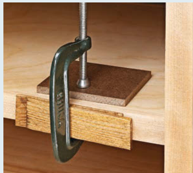
▲ For added pressure, apply small C-clamps to the panel, and drive in shims to hold the edging tight.
