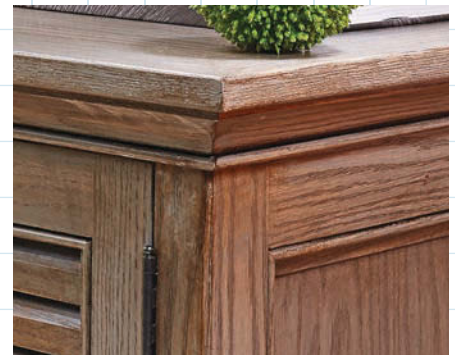
▲ Built-up moldings below the top and on the end frames help to give this functional storage project a fine-furniture look.
