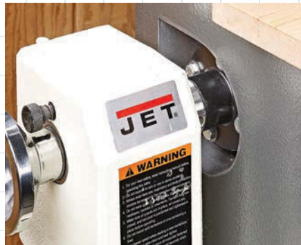
▲ Your lathe supplies power to the sander by using a dedicated faceplate mounted on the spindle.
