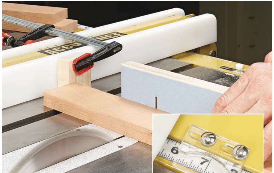
▲ A 1"-thick stop block positioned ahead of the blade provides clearance for the workpiece and makes setting the rip fence easy.
