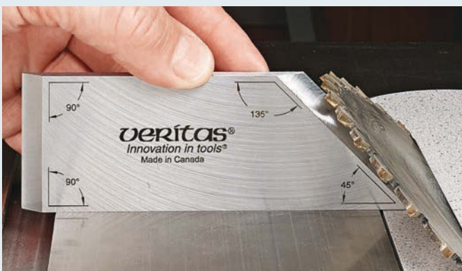
▲ The Veritas Blade Gauge is made from thick steel to help it stand on edge for checking blade angles. The ends are ground to a fine edge for accurate registration against the blade.
