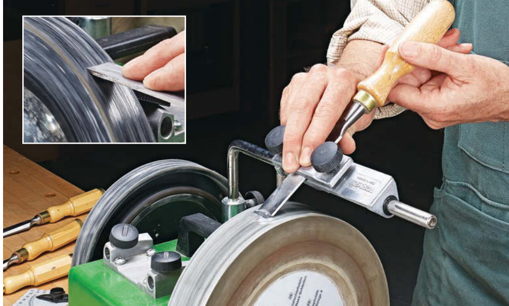
▲ The Tormek uses two wheels to sharpen all kinds of tools. A stone wheel spins in a water bath. This helps to keep the stone from clogging and cools the tool being sharpened at the same time. The leather wheel on the opposite end (inset) strops the edge to a mirror shine.
