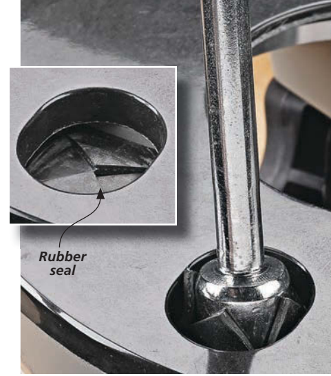
▲ Milwaukee routers incorporate a rubber seal to help keep dust out of the bit height adjustment mechanism.
