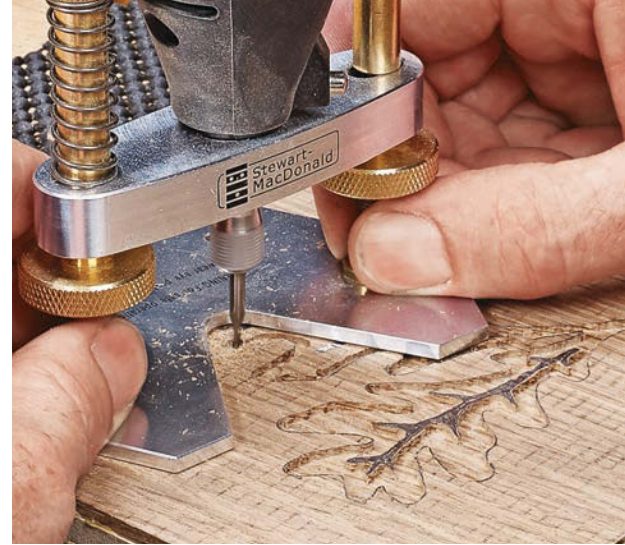
▲ Routing the recess for each metal piece is detailed work. Using a small bit gives you the best control and allows you to work into tight corners.
