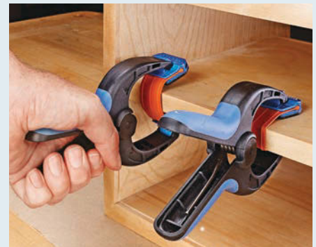
▲ These new Bandy Clamps from Rockler are handy tools for applying edging to plywood (refer to Sources, page 67).
