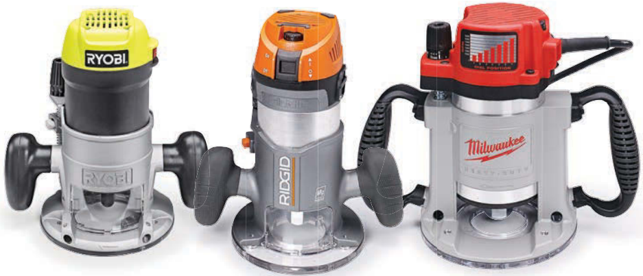
▲ Router motors vary in size from the entry-level 1.5-hp Ryobi R163GK to the 3.5-hp Milwaukee 5625-20 router. Mid-size routers, like the Ridgid R22002 , can handle most routing tasks in a router table and fall in the 1.75- to 2.25-hp category.
