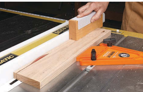
▲ A notched 2x4 push block is the simple solution for ripping edging strips. It keeps your fingers safe as you pass the block right over the blade.
