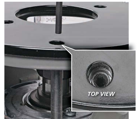
▲ Bosch routers locate the adjustment screw for the bit height right at the baseplate for easy access.
