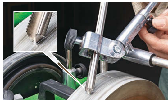
▲ Add-on specialty jigs let you put a perfect edge on hard-to-sharpen tools like turning gouges and carving tools.
