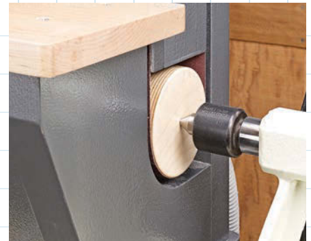
▲ A live center in the tailstock supports the opposite end of the drive roller for smooth operation.
