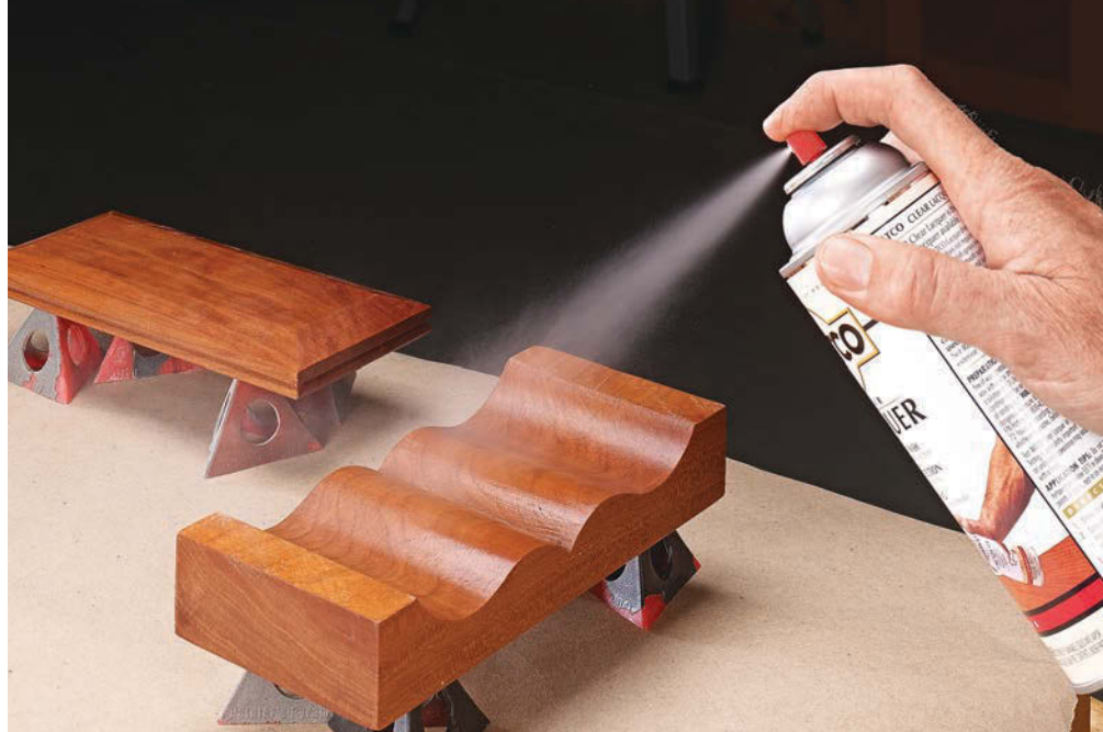
▲ Aerosol nitrocellulose lacquer dries quickly and offers moderate wear resistance. Plus, it imparts a smooth, amber tone that's desirable in many woodworking projects. I find that it's an excellent choice for the smaller, decorative projects that I make in my shop.
