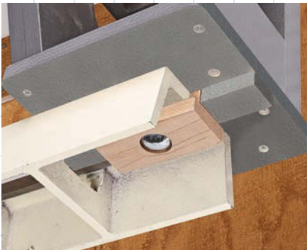
▲ The clamping block is an oversize, shop-made T-nut that fits between the ways on the lathe bed.
