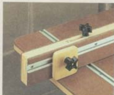
T-Track. Both the fence and the stop block ride in aluminum T-track. Toilet bolts and star knobs are used to lock them in place.
