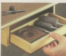
Storage Tray. A small, pull-out tray provides a convenient place for storing a chuck key, drill bits, or sanding drums.
