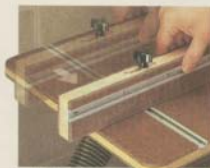
▲ Fence. Loosening a couple of knobs allows you to adjust the fence quickly or remove it entirely.
