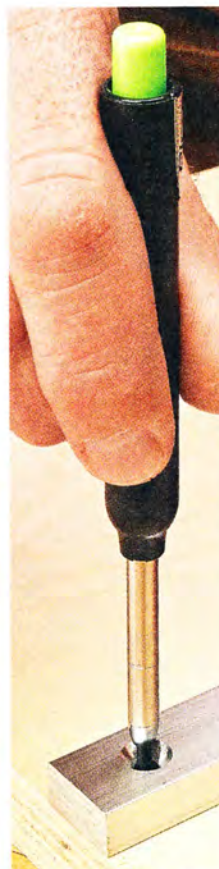
▲ Long-Nosed. The Pica-Dry specializes in marking in tight areas. The sharpener is built into the cap.
