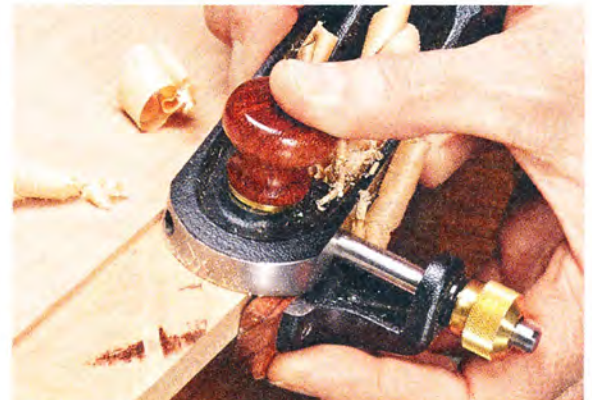
▲ Special Features. A rabbet plane cuts tight into a corner while the fence helps maintain the width of the bevel along the panel's edge.
