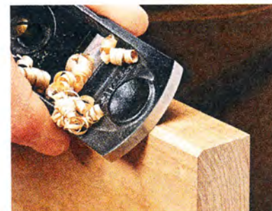
▲ Narrow Chamfers. A small block plane is ideal for creating eased edges on workpieces.
