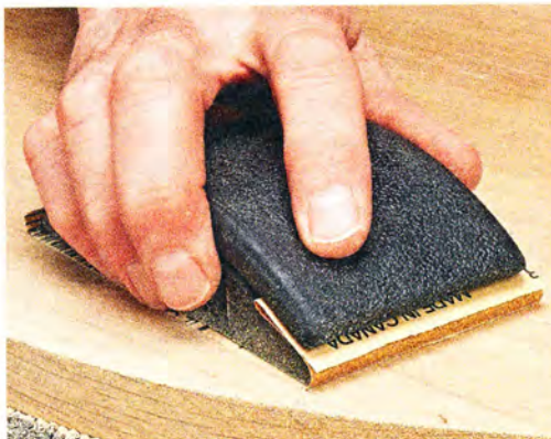
▲ Rubber Block. Dense rubber gives this block just the right amount of cushion. Slits in the ends securely grip the sandpaper.
