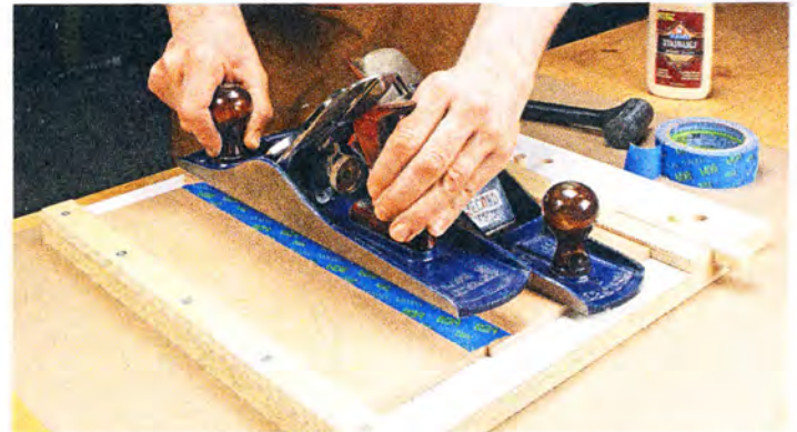
▲ Add Some Weight. A couple of hand planes keep the panel from cupping while the glue dries. Masking tape across the joint lines prevents glue stains on the planes.
