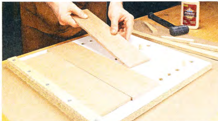
▲ Into the Clamping Jig. Lay out the boards on the clamping jig. After applying a thin bead of glue to the mating edges, set the loose clamp bar in place.
