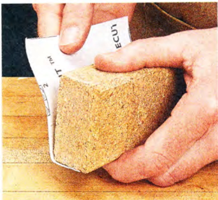
▲ Cork Block. Using adhesive-backed sandpaper means you don't need to hold the paper to the block.
