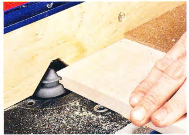
▲ Face Down. Rout the first part of the joint with the inside face of the workpiece down on the router table. A backer board prevents tearout.
