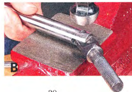
▲ Lock It Down. You'll need to locate the centerline of the table locking stud first (A), then pin the shaft to the locking handle stud (B). Finally, clamp the locking shaft bearing block in place and screw it to the table (above).
