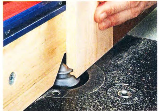
▲ On End. The mating part of the joint is cut with the workpiece held vertically against the fence. The backer board helps keep it square.
