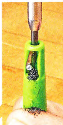
▲ Long-Nosed. The Pica-Dry specializes in marking in tight areas. The sharpener is built into the cap.
