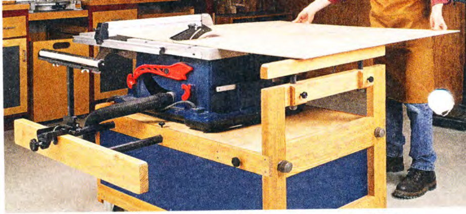
▲ Solid Support. Raise the side support flush with the saw table and extend the outfeed support to effectively increase the working size of a benchtop table saw. The result is safer and more accurate cuts.
