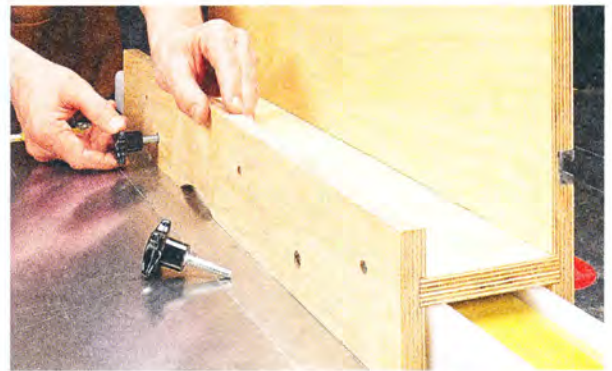
▲ Threaded Inserts & Knobs. For a fence that will see lots of action, it's worth going to the trouble of installing threaded inserts and knobs.
