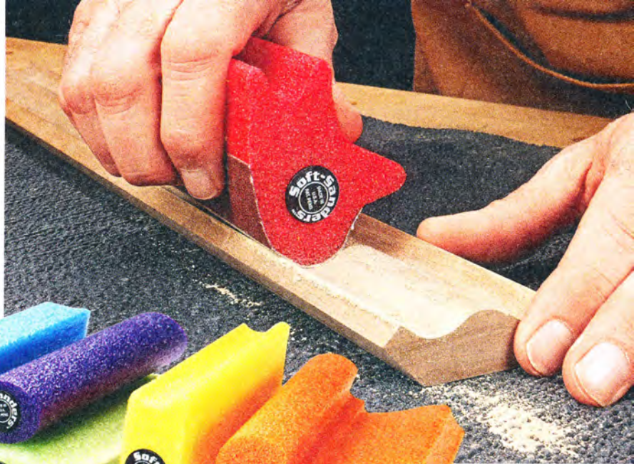
▲ Profile Blocks. Each block features several profiles, so you can find one that matches the workpiece.
