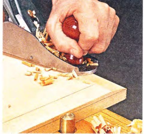
▲ End Grain First. Skew the plane slightly as you slice off the end grain. Then work on the long-grain edges.
