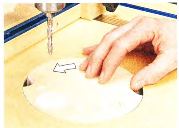
▲ Solid Support. The insert is offset from the centerline of the bit. To provide solid backing for a new bit, simply rotate the insert to a fresh area.
