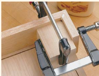
▲ Clamping blocks hold the corners square when test-fitting the miters and gluing the aprons together.
