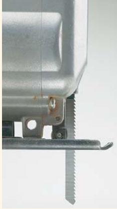
▲ To prevent chipout on the top face of plastic laminate, I use a special reverse cut sabre saw blade. (The teeth point down.)
