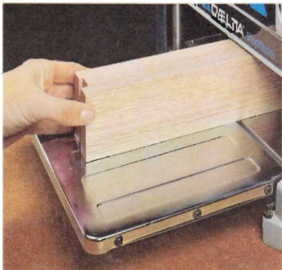
▲ Planing Multiple Pieces. By grouping several narrow boards together, you can plane them all to exactly the same width at the same time.
