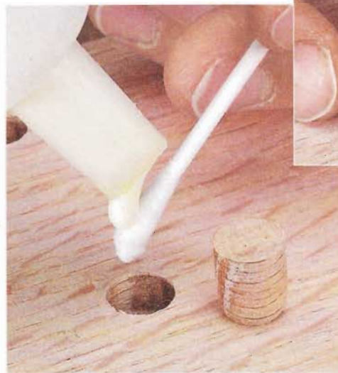
▲ Match Plugs & Glue. Choose a plug with grain and color that's a good match with the surrounding wood (inset). Glue it in with a small dab of glue.
