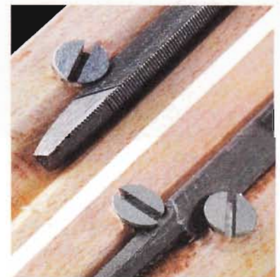
▲ Attach File. Position the screws to trap both ends of the triangular file to hold it securely in place on the block.
