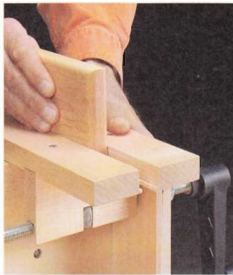
▲ File The Teeth. Forming a tooth to the exact depth should take about four strokes. Always file on the push stroke.
