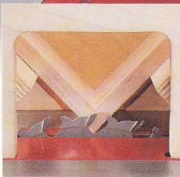
▲ Depth of Cut. The "window" in the jig makes it easy to set the depth of cut across the corner.
