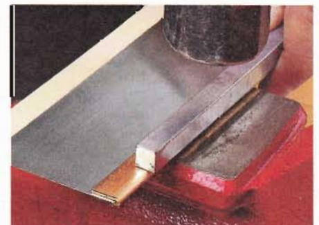
▲ Crimp the Back. Finally, use the hammer and bar to crimp the brass back around the blade for a snug fit.
