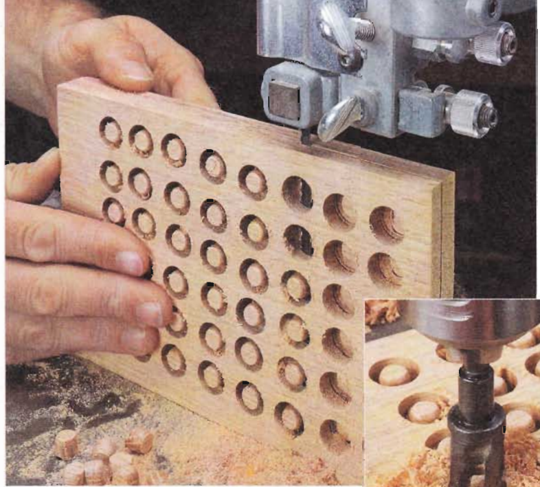
▲ Create The Plugs. Make plenty of plugs from some scrap material used on the project (inset). Then cut them free at the band saw.
