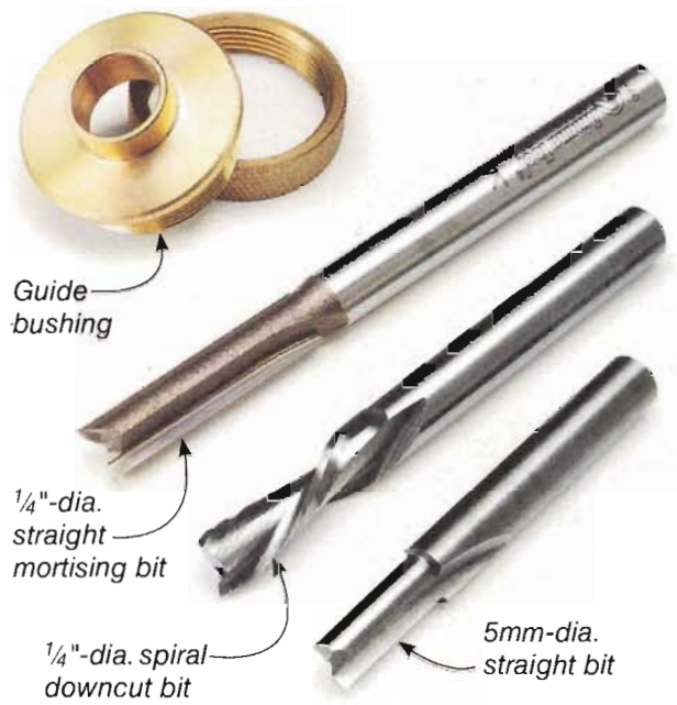
▲ Stopped Holes. Set your plunge router to drill holes to half the thickness of the workpiece.
