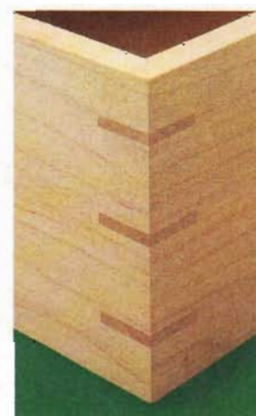
▲ Low-Key Look. Installing splines made from the same material as the box provides a subtle detail.
