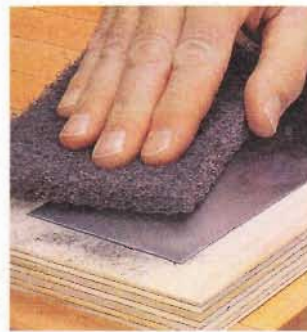
▲ Clean Up. After filing away the rough edges, sand the bluing from the entire blade.
