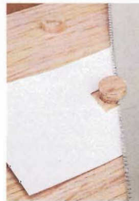
▲ Match Plugs & Glue. Choose a plug with grain and color that's a good match with the surrounding wood (inset). Glue it in with a small dab of glue.
