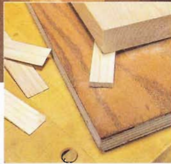
▲ Face Joint. By supporting a workpiece with a sled and several shims, it's possible to flatten the face of wide stock that's bowed or warped using a planer.
