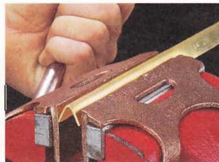
▲ Bend It Flat. Clamp the folded back in the vise and bend it until it's almost flat. Jaw liners protect the brass from marks.
