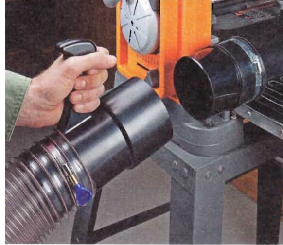
▲ Sturdy Handle. The large handle fits not only the dust collection ports of most tools, but all the attachments as well.
