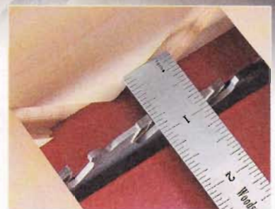
▲ Kerf Location. To locate the kerf, just measure from the inside face of the jig to the saw blade.
