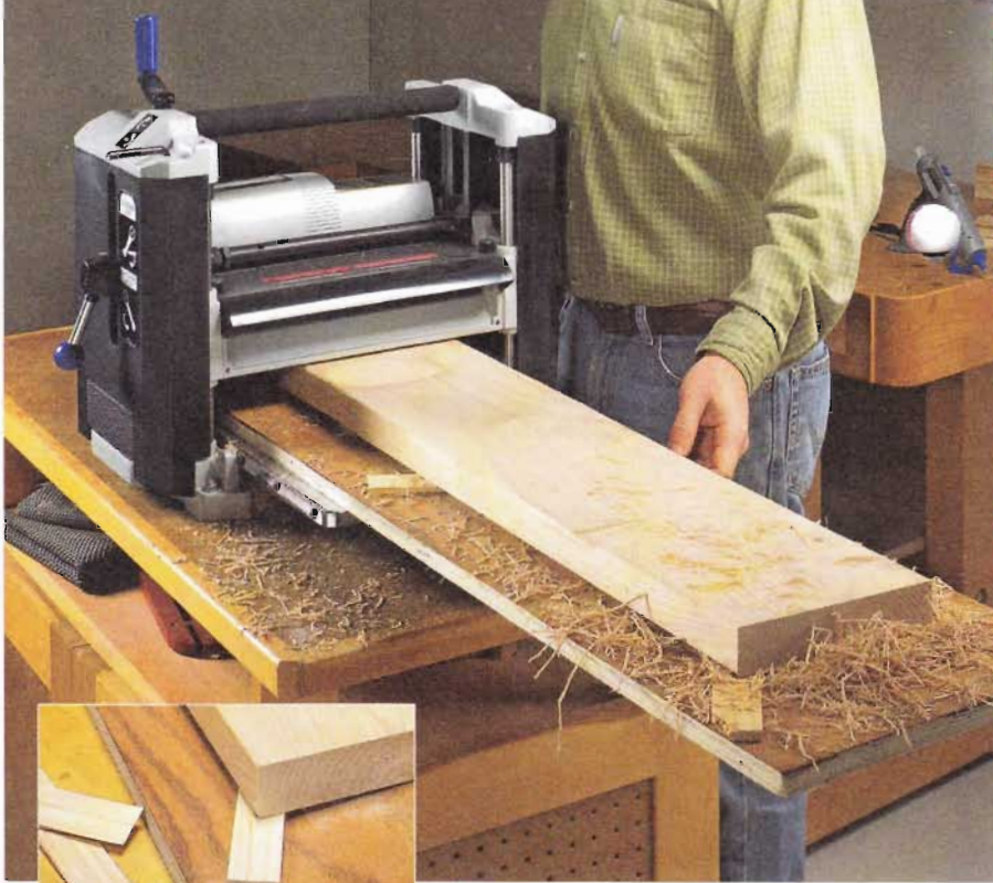
▲ Face Joint. By supporting a workpiece with a sled and several shims, it's possible to flatten the face of wide stock that's bowed or warped using a planer.
