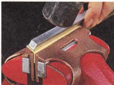
▲ Initial Bending. Use a hammer and a piece of steel to gradually bend over the back in a vise, a small section at a time.
