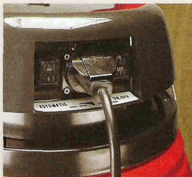
▲ The "Brains." Switched to auto mode, the vacuum powers up automatically when you turn on a tool.
