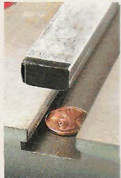
▲ Give the Runners a "Lift." A penny at each end of the metal runner raises it just enough to clear the top of the saw table and contact the base of the sled.
