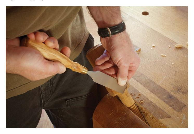
Slice while paring. It's usually best to use a slicing cut while paring. Move the chisel both forward and laterally to do this. My left hand is moving the chisel to my left.
