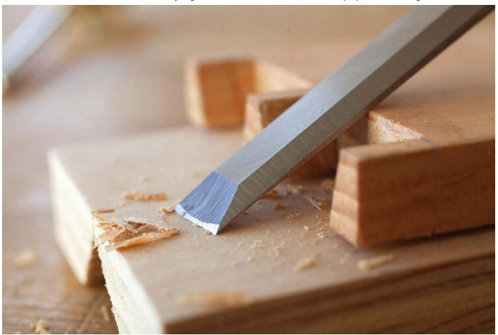
A low-angle chisel. This low-angle chisel is great for the final chop when dovetailing. It's fussy. But some customers pay for fussy.
