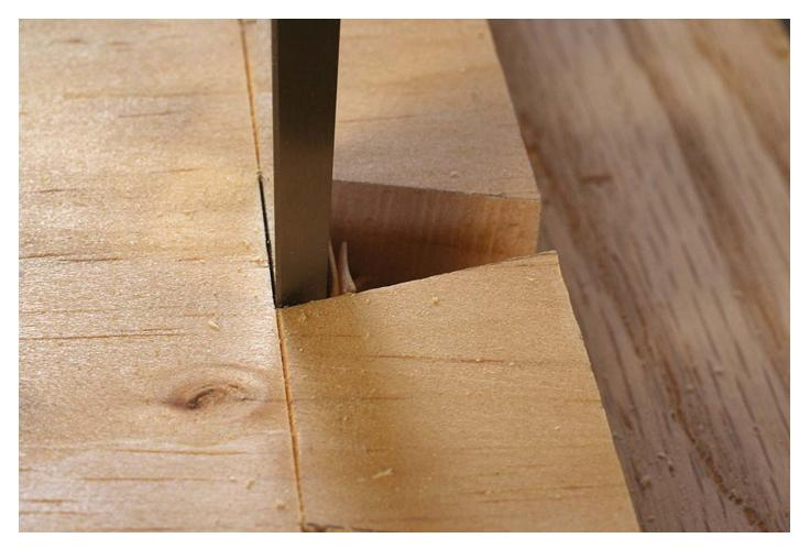
Then remove half of the remaining waste. Continue this cycle until you cannot remove any waste. That's when you drop your chisel tip into your baseline.
