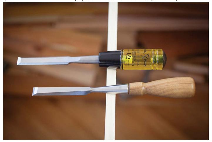
Handle-heavy hurts. If the balancing point for the tool is in the handle, I think it's too heavy for light chopping. Cut the handle down or replace it with a wooden one.
