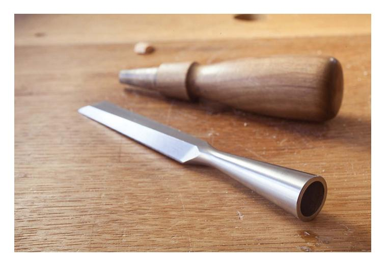
Instant butt chisel. Removing the handle of your socket chisel gets you into most tight spaces.
