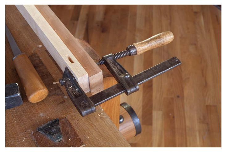
A solid mortising setup. This is a fairly common English way to cut mortises. Note that the side pressure from the cramp, I mean clamp, helps prevent the work from splitting during mortising.
