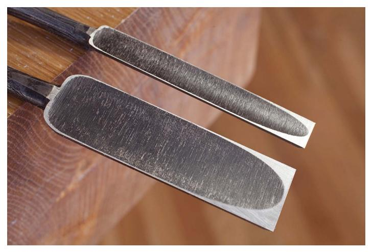
That's not flat. One of the nice features of Japanese chisels are the hollows ground in the back. These hollows make the chisel easy to set up – there's less steel to flatten.
