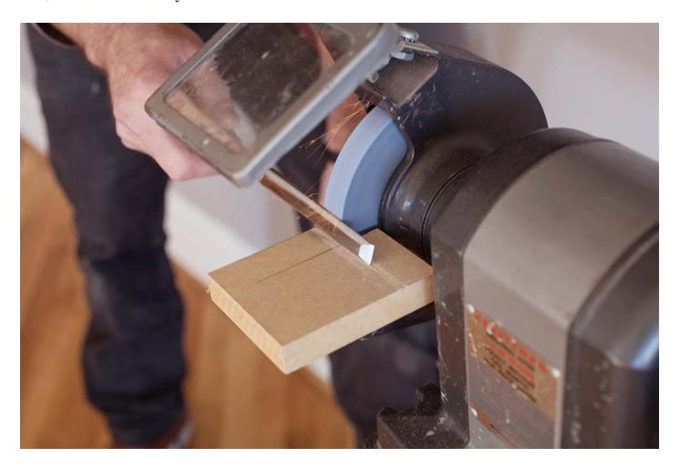
Remove metal & tedium. Grinding out a bellied back can save hours of work. Once again, a flat platform around the wheel makes this operation a cinch.
