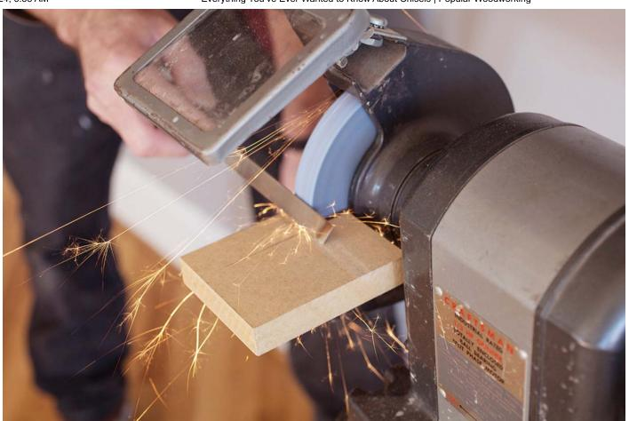
It's not scary. If you have a flat platform around your grinding wheel, then grinding down the side bevels is easy work, even for a beginner.
