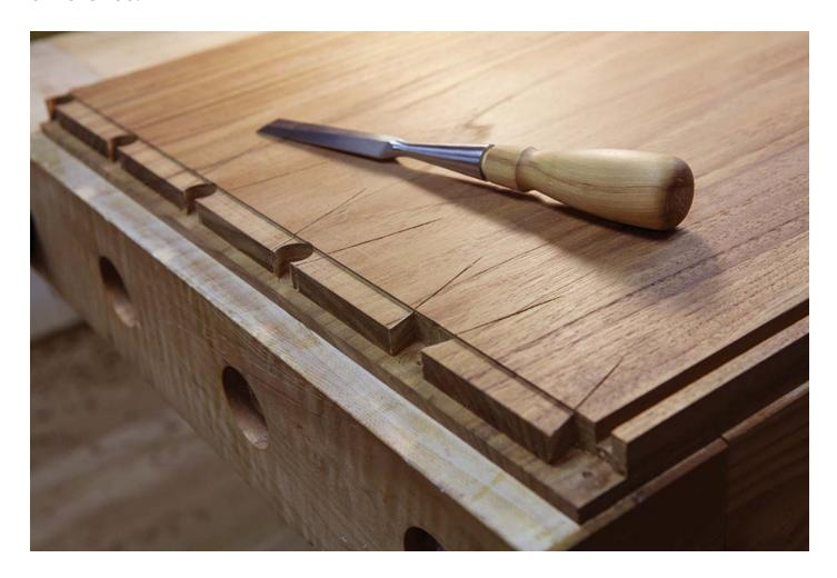
Chop, hone, repeat. When dovetailing a carcase, I hone my chisel after each corner. When dovetailing a large drawer, I might do two corners before honing. With small drawers, I hone after finishing each drawer. These little rules keep me sharp.
