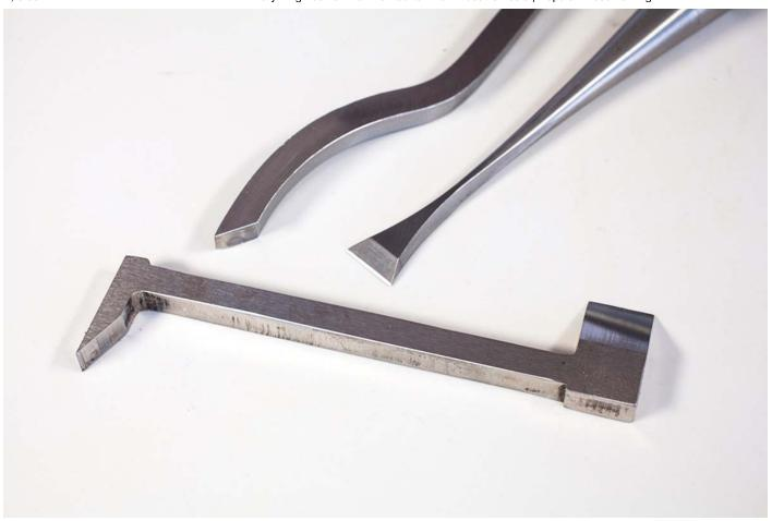
Second-string chiselers. The fishtail chisel (top, right) is a huge help when cleaning up half-blind dovetails. The swan-neck chisel (top, left) scours the bottom of mortises. And the drawer-lock chisel (sorry, no cute animal name) lets you work in tight quarters.
