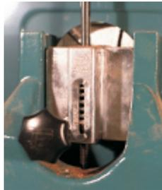
The tension scales on most bandsaws are inaccurate. It's common for scales to indicate a tension far above the actual tension on the blade.
