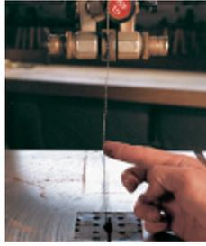
If you don't have a tension meter, you can roughly tension the blade by eye. Raise the guides about 6 in. off the table and push the blade. The blade should deflect no more than 1/4 in.
