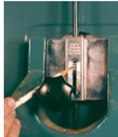
On a small consumer-grade bandsaw, I tension a 1/2-in. blade for resawing by almost completely compressing the tension spring.
