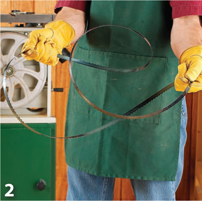
Extend your arms away from your body and spread your hands apart as you continue to uncoil the blade. As the coils straighten out, the blade will spring into one big loop, so don't be startled. 🍀
