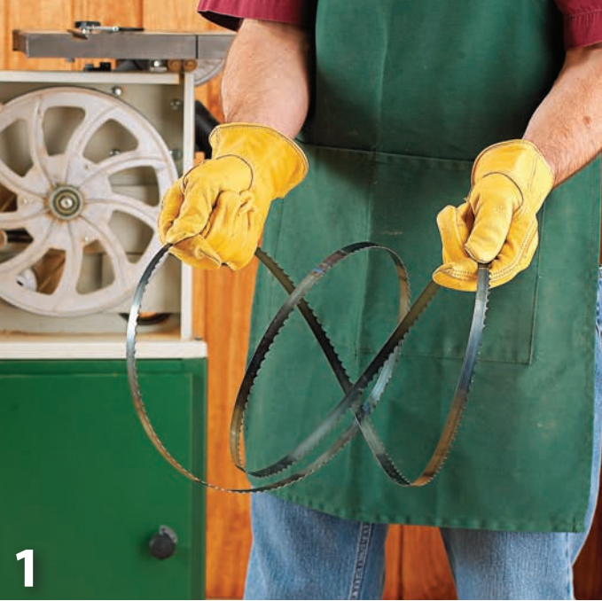
After removing the clip or masking tape, hold one outside blade coil in each hand with the teeth pointed away from you, and slowly spread them apart. Keep your hands low to protect your face from the blade.
